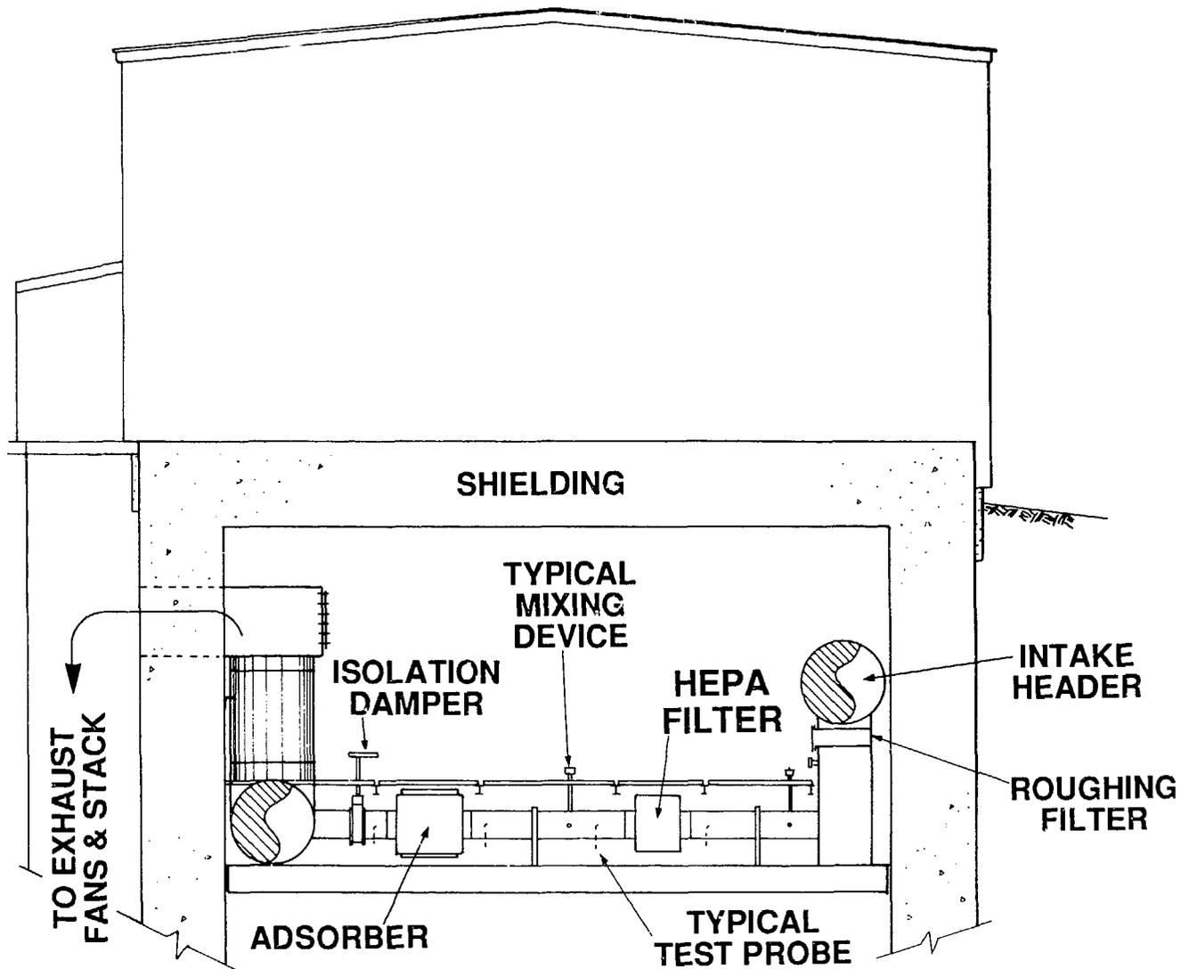
**FIG. 3 EFS BUILDING SECTION**
