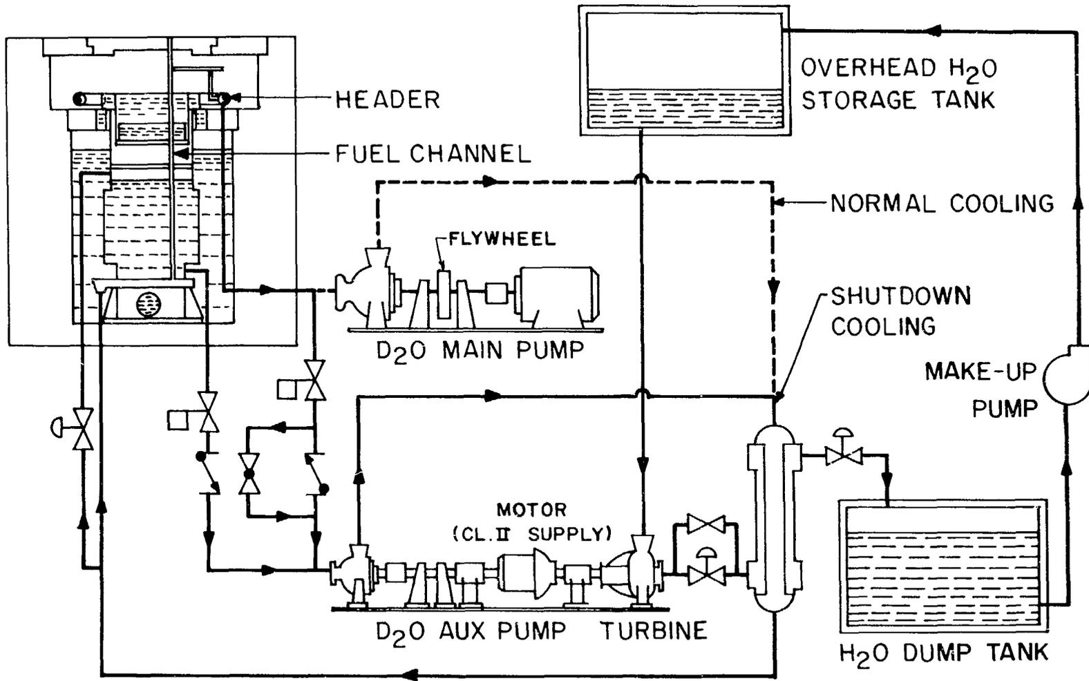
Fig. 5 SHUTDOWN COOLING SCHEMATIC
