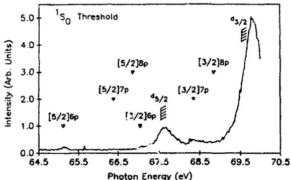
Figure 3:  $1S_0$  Threshold spectrum in Xe
