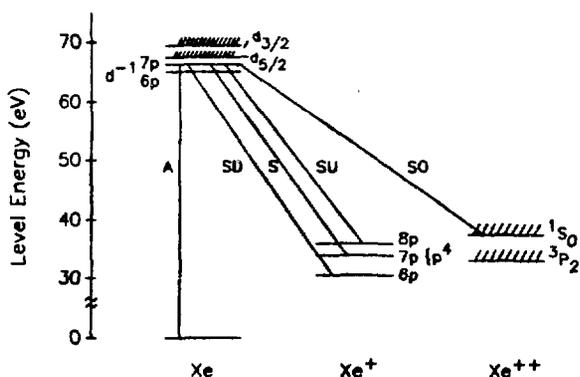
Figure 2: Energy Level Diagram for Xe
