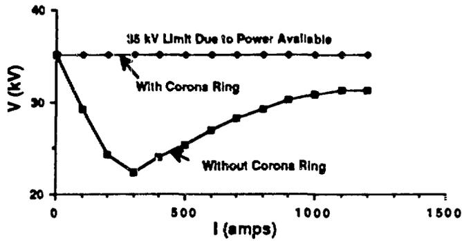
Fig. 2. Voltage standoff vs magnetic field current.
