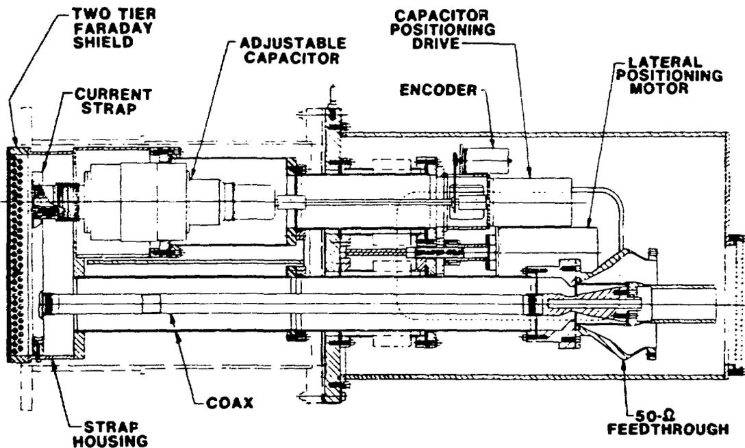
Fig. 1. Sectional view of the ORNL compact resonant loop antenna.
