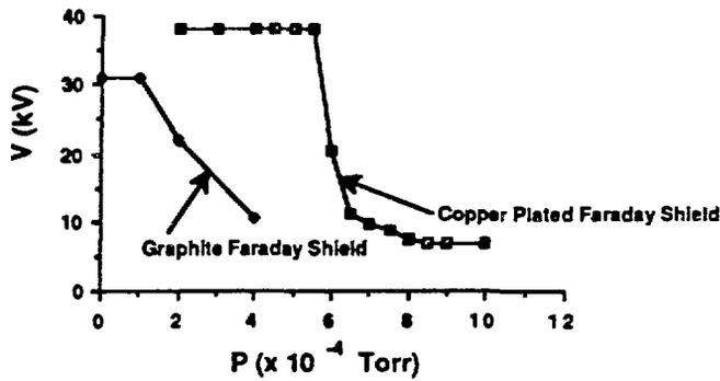
Fig. 3. RF voltage holdoff vs pressure.
