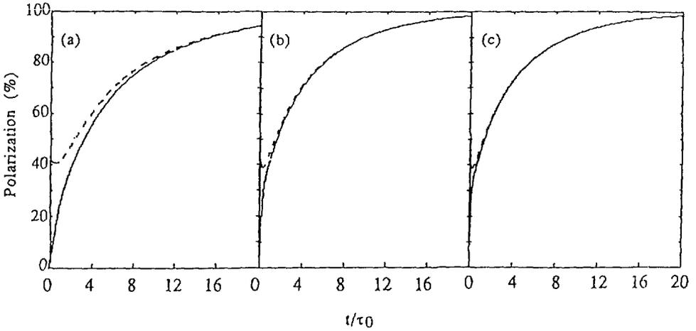
Fig. 2. Time dependence of the polarization of protons.  $\tau_0(= A_{12})$  means the life time of the excited state. Figures (a),(b) and (c) are at the transition probabilities of  $A_{12}$ ,  $5A_{12}$  and  $10A_{12}$ , respectively. The solid lines refer to the ionization of beam atoms from both ground and excited states with a foil, the dashed lines from the excited state only with the laser ionization injection.
