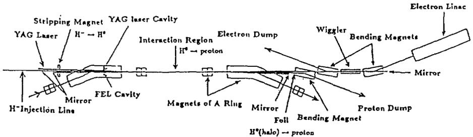
Fig. 3. Injection scheme by a FEL and YAG laser. The FEL system consists of an electron linac, two bending magnets, a wiggler and two mirrors. The electron beam, which is deflected by the magnet, passes through the wiggler which radiates photons. The photons are accumulated in the cavity between the two mirrors and excite the hydrogen atoms in the several meter interaction region. The excited hydrogen beam is ionized by the light in the YAG laser cavity.
