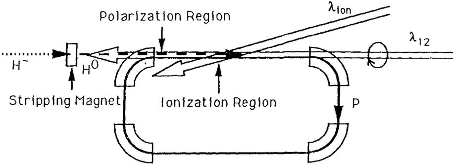
Fig. 1. The  $H^0$  beam(dashed line) is excited and polarized by the laser with a wavelength of  $\lambda_{12}$  in the polarization region. Then, it is ionized with simultaneous irradiation by another laser ( $\lambda_{ion}$ ) in the ionization region.
