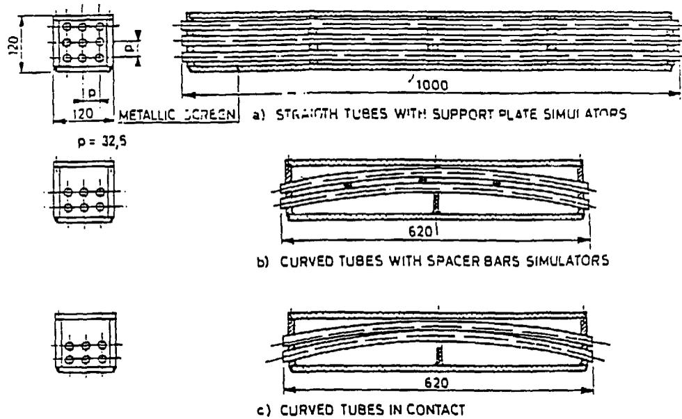
Fig. 1 - Sealed boxes for blind tube inspection.
