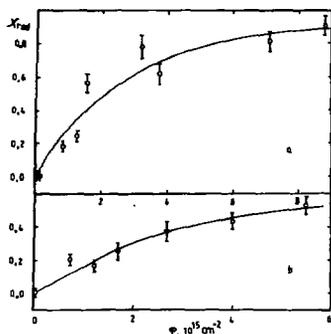
Fig. 5. The yield  $X_{\text{rad}}$  in the blocking minimum  $\langle 101 \rangle$  of diamond versus ion fluence: 25 MeV  $^{40}\text{Ar}$  (a) and 122 MeV  $^{129}\text{Xe}$  (b).
