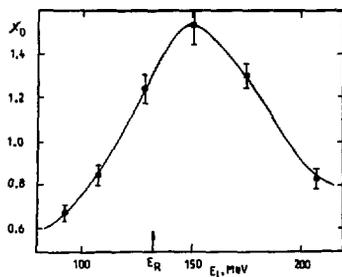
Fig. 3. Relative yield  $X_0$  of recoils along the Si  $\langle 111 \rangle$  axis, oriented at  $53^\circ$  to the  $^{40}\text{Ar}$  beam, as a function of projectile energy.  $E_R$  is the grazing energy.
