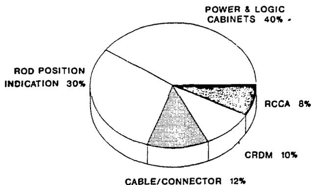
Figure 2 CRD System Failures
