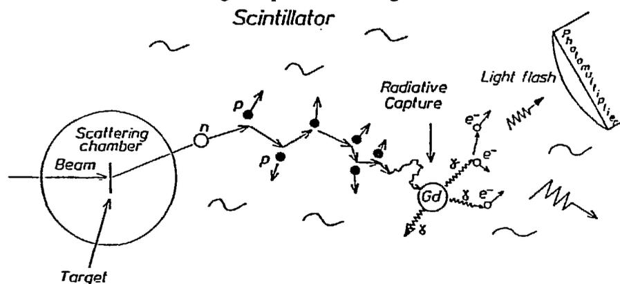
Fig.1 Scheme for neutron detection in Gd loaded, liquid scintillator detectors.
