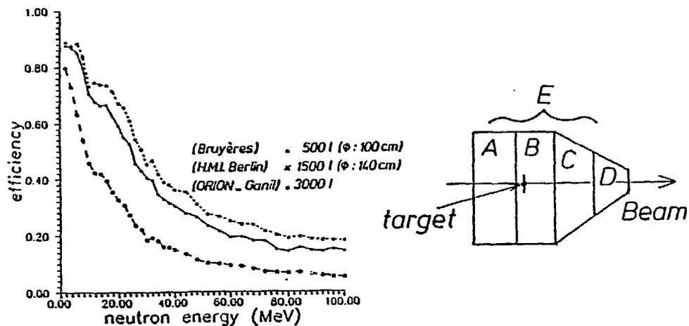
Fig.2 Detection efficiency computed as a function of kinetic energy for neutrons emitted isotropically in three detectors used at GANIL. The geometry of ORION is also schematized.
