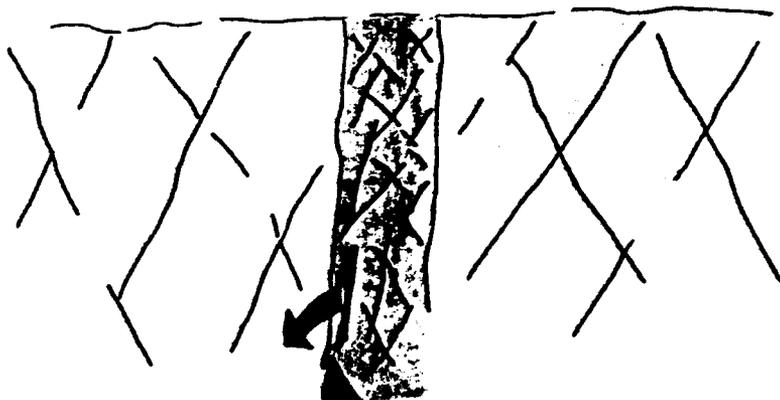
Figure 4.9.4 Tension zone with blocky-partly crushed rock. Considerable local leakage.
