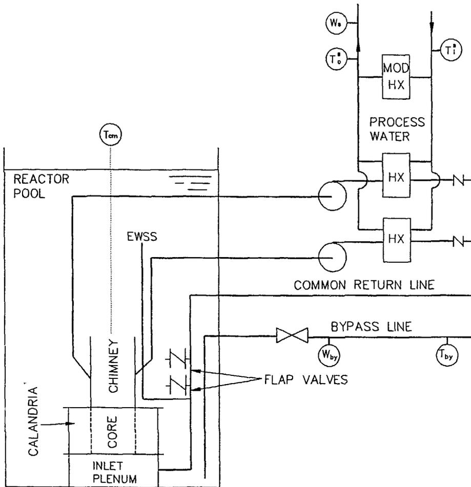
Fig. 1. KMRR Coolant Flow Schematics and Thermal Power Measurement System
