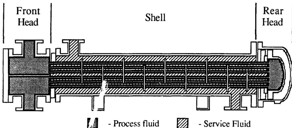
Figure 1: Cross-section of a Typical Shell-and-Tube Heat Exchanger
