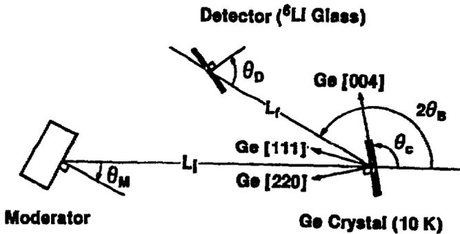
Figure 6. Time Focussed Crystal Spectrometer arrangement for measuring the emission time distribution as a function of wavelength
