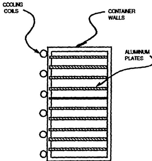
Figure 3a. The KENS internal cooling system for solid methane.
