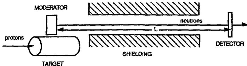
Figure 4. Arrangement for measuring the wavelength spectrum of a pulsed source moderator.
