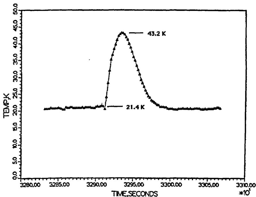
Figure 14. The temperature at the center of the IPNS "C" moderator as a function of time after an externally induced "burp".
