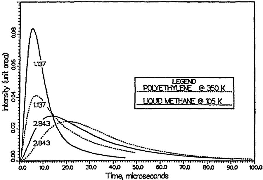
Figure 9. Pulse shapes at two wavelengths for an ambient temperature polyethylene moderator poisoned with .5 mm Cd, 22 mm beneath the viewed surface, and for a liquid methane moderator, poisoned 17 mm beneath the viewed surface.
