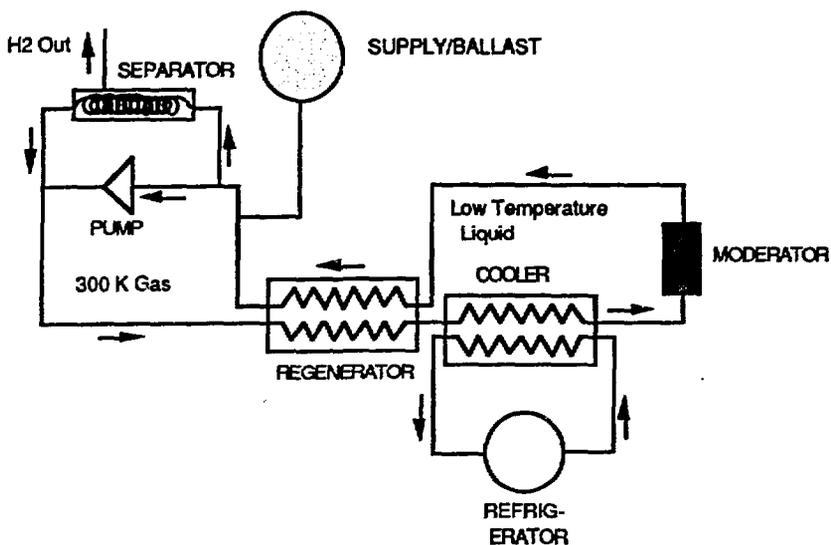
Figure 2b. Recirculating liquid-gas system.
