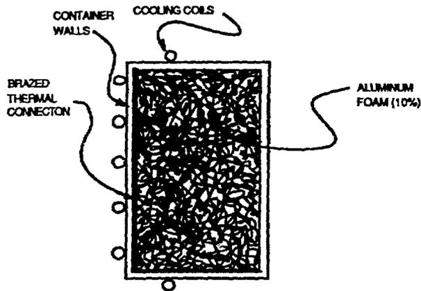
Figure 3b. The IPNS internal cooling system for solid methane and liquid Hydrogen.
