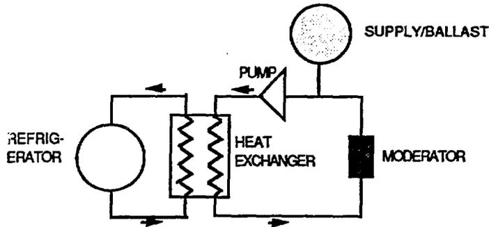
Figure 2a. Recirculating liquid system.
