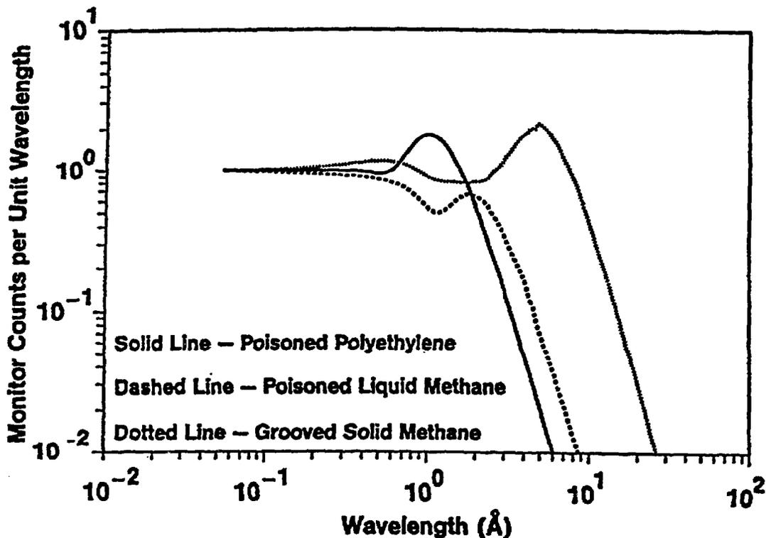
Figure 5. Comparison of flux spectra for 350 K polyethylene, 105 K liquid methane and 20 K grooved, solid methane.
