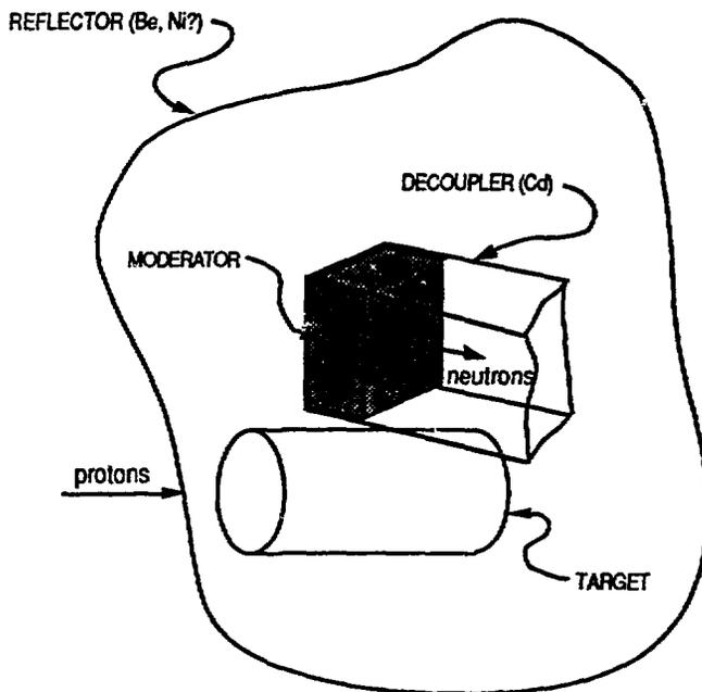
Figure 1. A typical arrangement of a target, moderator and reflector in a pulsed spallation neutron source. Targets are around 20 cm in length and 10 cm in diameter; moderators dimensions are about 5x10x10 cm.
