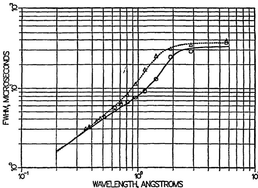
Figure 10. The Full Width at Half Maximum of pulses from a poisoned ambient temperature polyethylene moderator and from a poisoned liquid methane moderator, vs wavelength. The curves are physically-motivated rational polynomials fitted to the data.
