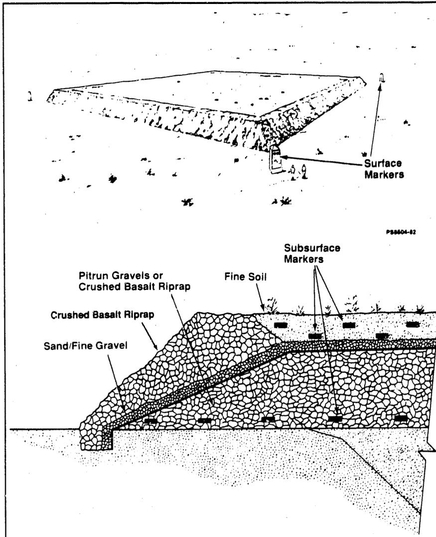
Figure 1. Typical protective barrier and warning marker system.
