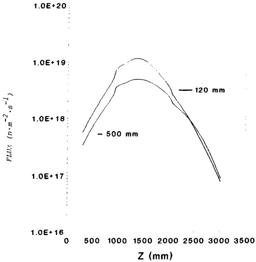
Figure 4: MAPLE\_D<sub>2</sub>O Axial Thermal Flux Distributions at 50 MW
