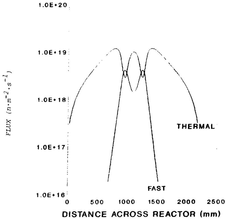
Figure 3: MAPLE\_D<sub>2</sub>O Radial Neutron Flux Distributions at 50 MW
