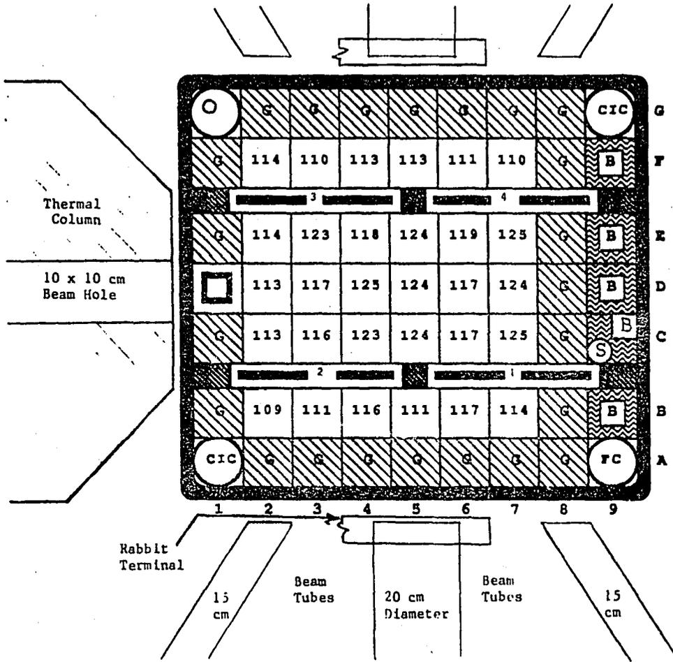
Figure 4: Typical 30 element HEU core
