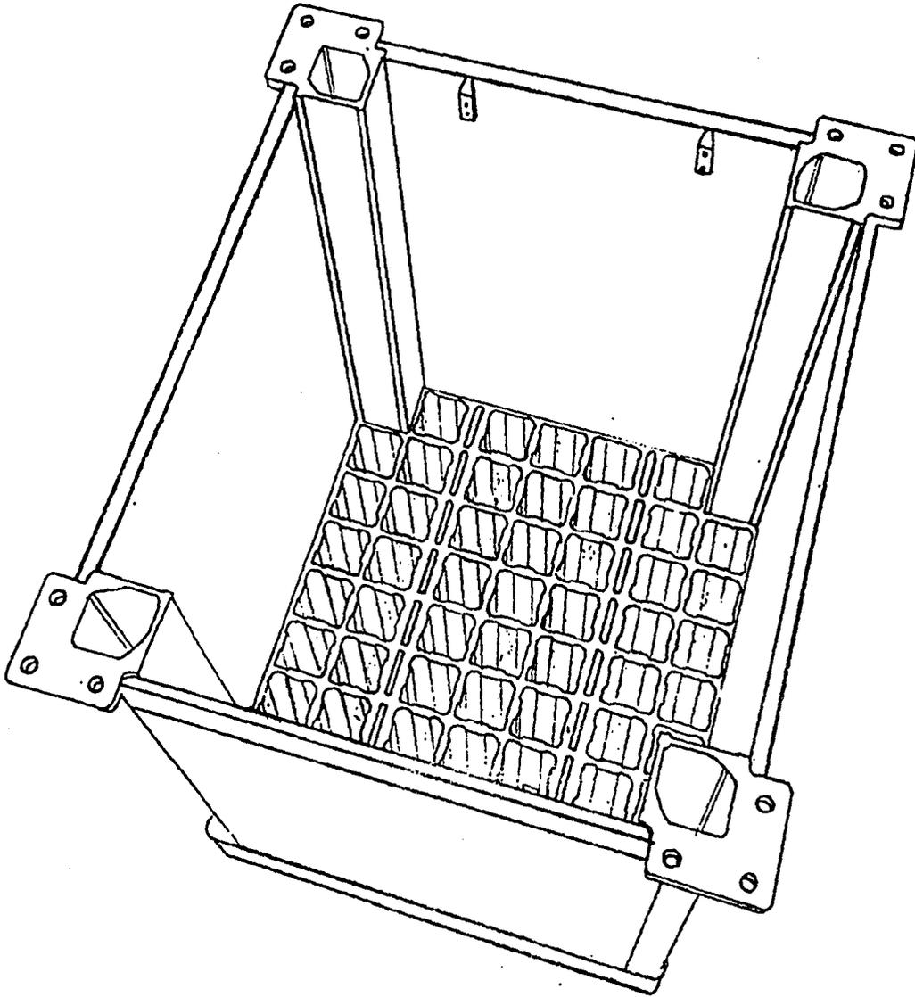
Figure 2: Reactor Core Grid Box
