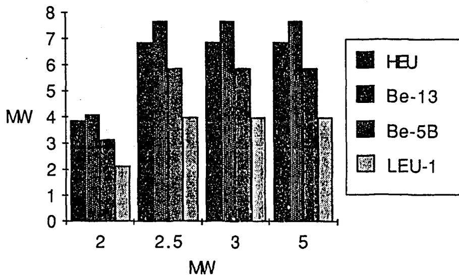
Figure 11: Power Level vs Onset of Nucleate Boiling
