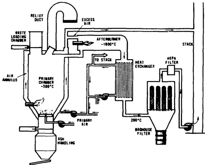
FIGURE 1: SCHEMATIC DIAGRAM OF CRNL STARVED-AIR INCINERATOR
