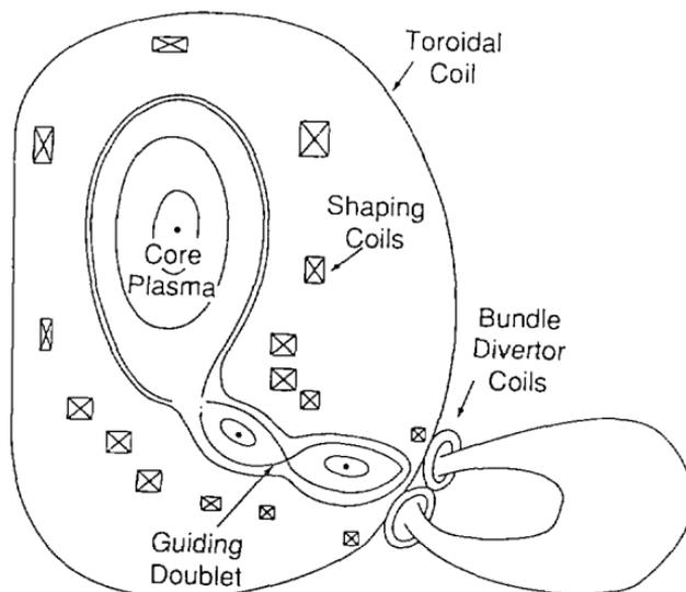
**Fig. 4 An example of the tokamak divertor configuration, which allows high temperature divertor operation.**
