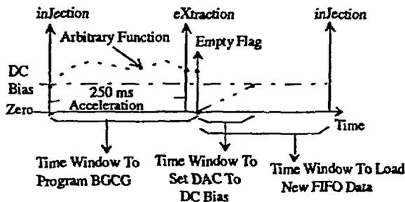
Figure 3. Arbitrary Function Timing in a Synchrotron Cycle
