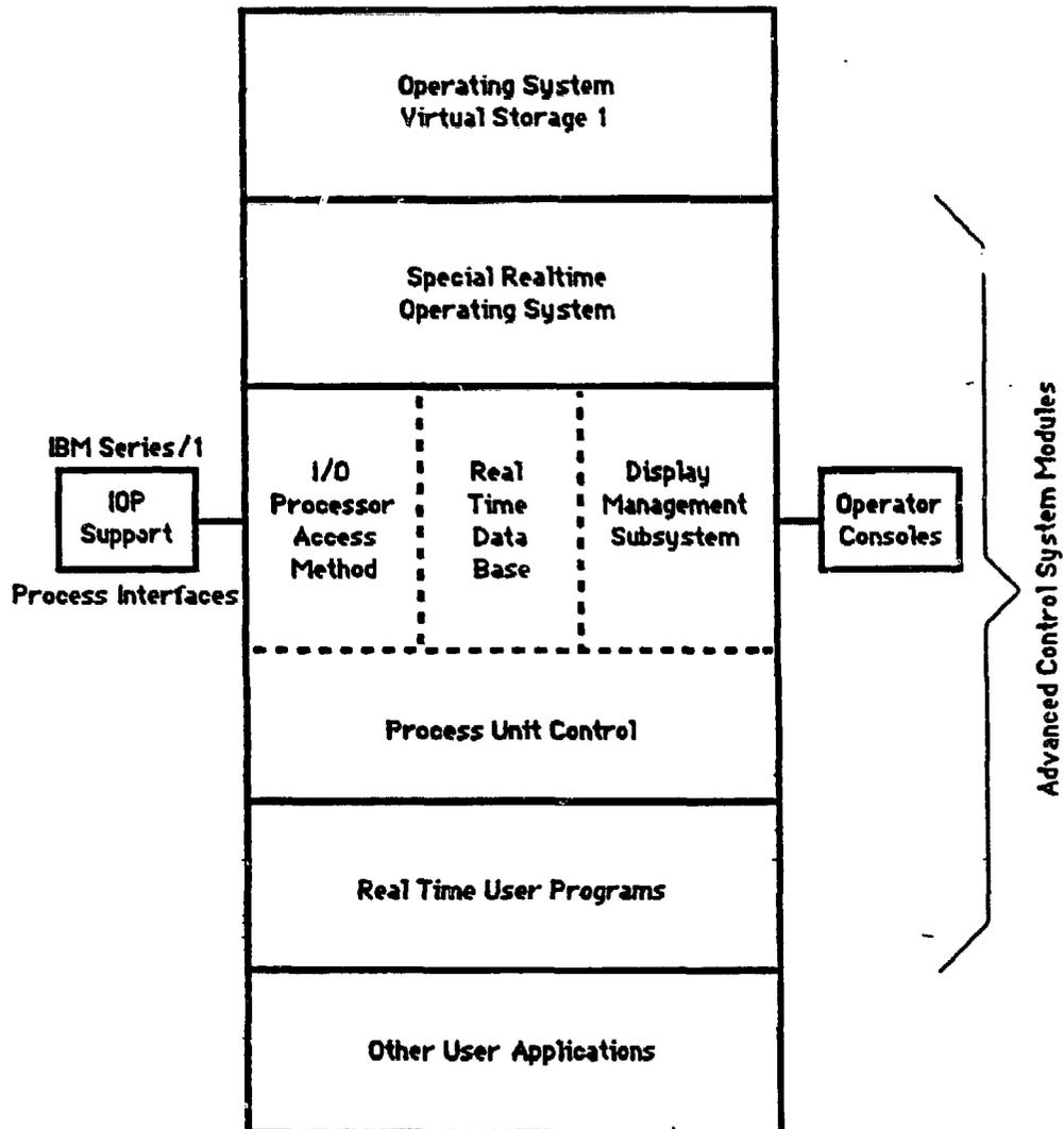
Fig. 3 : IBM Advanced Control System Schematic.
