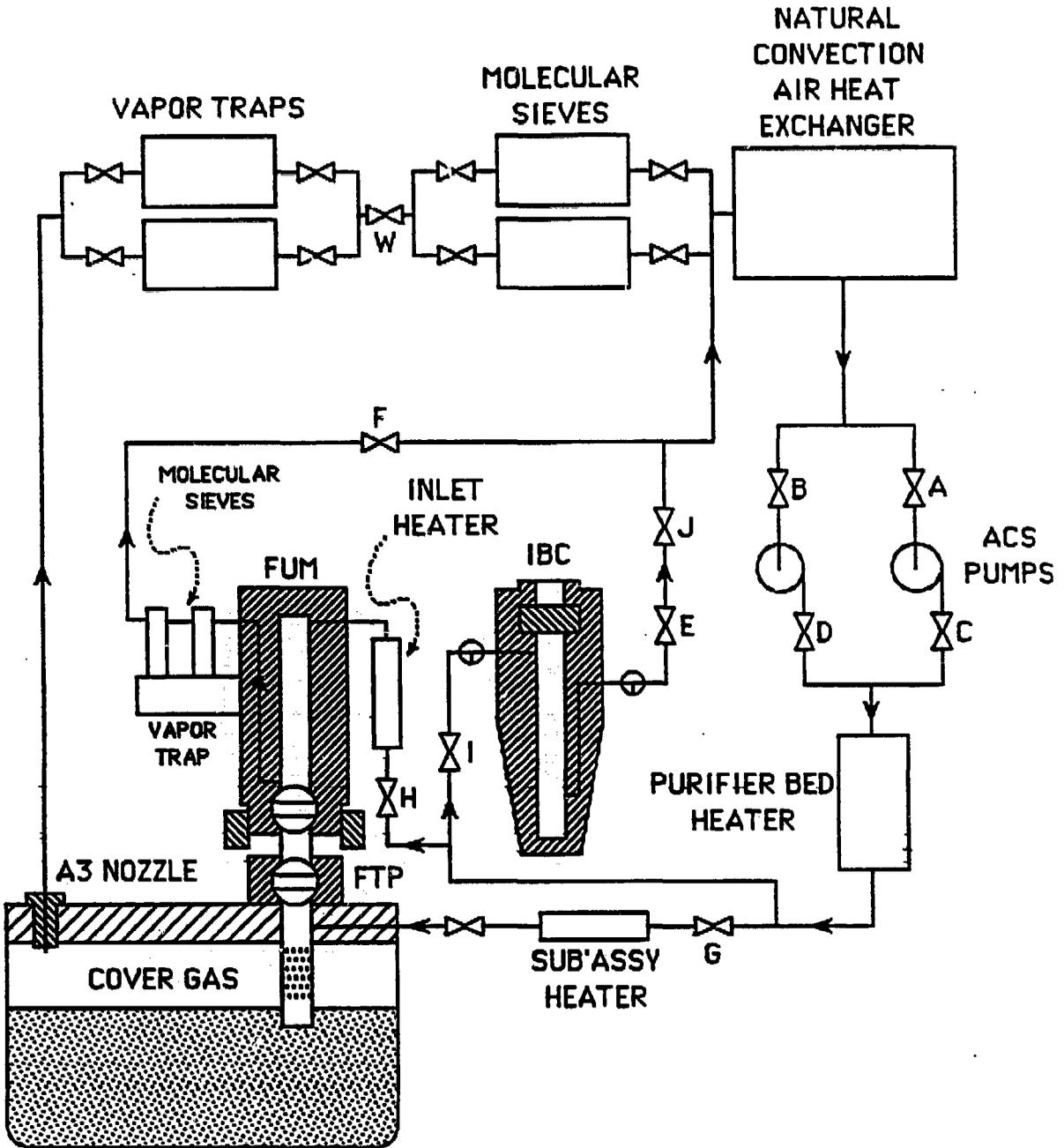
FIGURE 1: EBR-II ARGON COOLING SYSTEM FOR FUEL HANDLING
