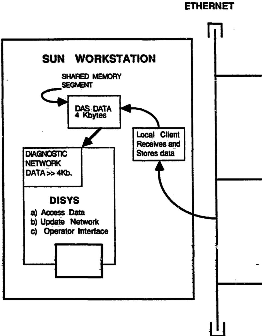
**FIGURE 5: DISYS ACCESS TO PLANT DATA THROUGH UNIX SHARED MEMORY SEGMENT**
