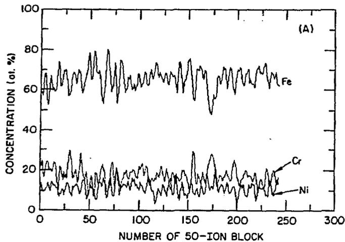
Fig. 3. Results of FLAP Analysis of the Shippingport PWR Pump Volute (Table 1) Showing Spinodal Decomposition and Ni-Si and Ni-Mo-Si Clustering in Ferrite; (A) Fe, Cr, Ni Profiles; (B) Ni, Si, Mo Profiles of (A); and (C) Profiles Similar to (B), Obtained from Another Ferrite Grain of the Same Specimen.
