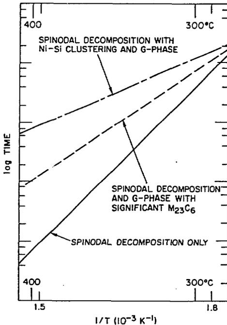
Fig. 4. Schematic Diagram of Relative Kinetics to Produce a Constant-Impact-Energy Drop for Three Hypothetical Cases of Metallurgical Transformation under Otherwise Identical Conditions. (A) Spinodal decomposition only (in ferrite), (B) Ni-Si clustering followed by G-phase precipitation plus (A), (C) significant M<sub>23</sub>C<sub>6</sub> precipitation on austenite/ferrite boundary during aging plus (B).
