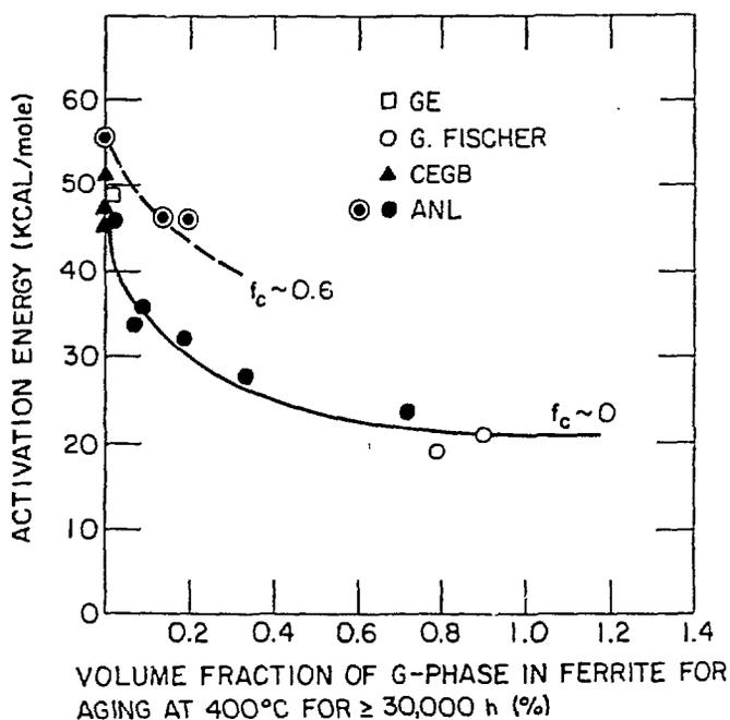
Fig. 2. Activation Energy of Aging versus Volume Fraction of G-Phase in Ferrite Observed after Aging at 400°C for  $\geq 30,000$  h.  $f_c$  in the figure denotes fraction of the ferrite/austenite boundary covered by  $M_{23}C_6$  carbide.
