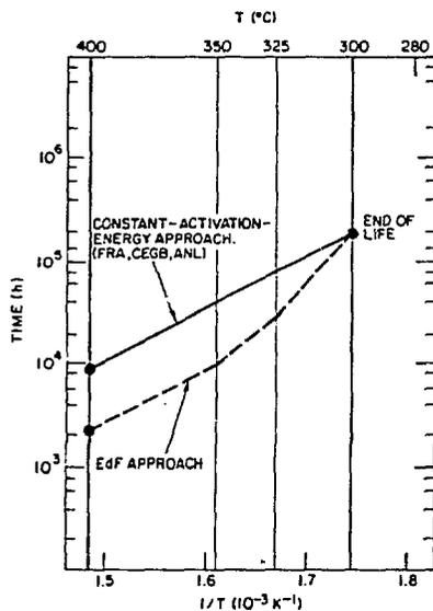
Fig. 1. Schematic Illustration of Selecting Accelerated Aging Conditions Based on Single and Multiple Activation Energies of Aging.
