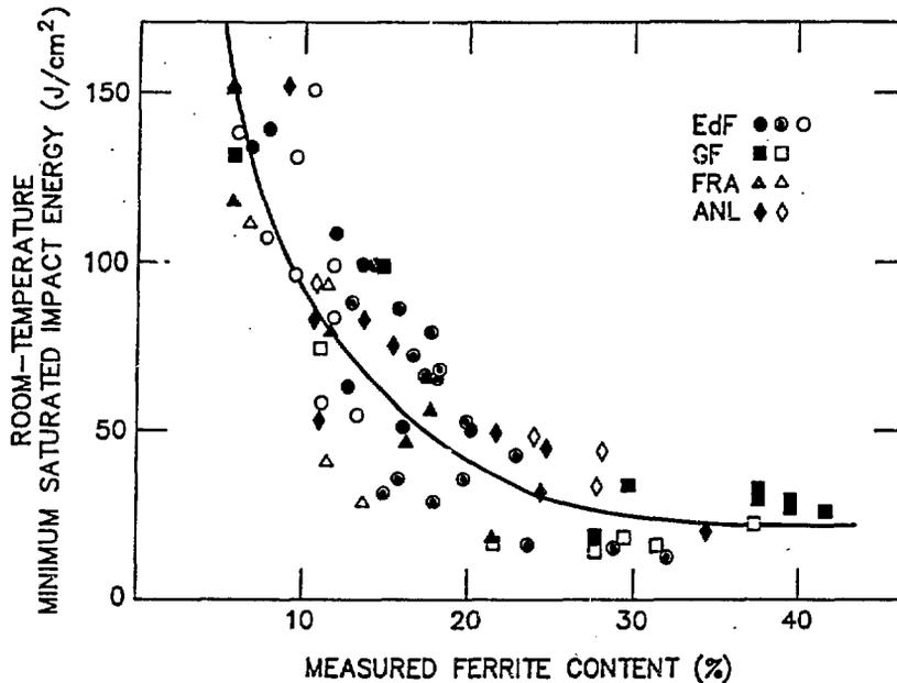
Fig. 6. Room-Temperature Saturated Impact Energy vs. Measured Ferrite Content Plotted for Heats Reported in Refs. 1 (GF), 4 (FRA), 17 (EdF), 26 (ANL), and 30 (ANL).
