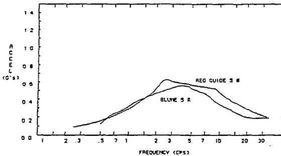
Fig. 7 COMPARISON OF REG GUIDE AND BLUME SPECTRA
