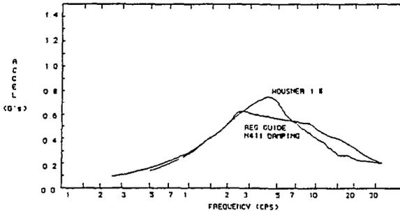
Fig. 8 COMPARISON OF HOUSNER 1% SPECTRA WITH REG GUIDE H-411 SPECTRA
