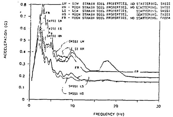
Fig. 9 COMPARISON OF SASSI AND FREDAs 5% N-S SPECTRA - ELEV 0'
