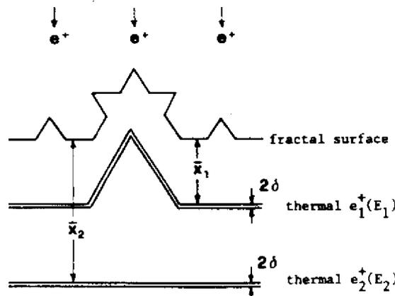
Fig.1 Schematic positron of  $e_1^+(E_1)$  and  $e_2^+(E_2)$  ( $E_2 > E_1$ ,  $\bar{x}_2 > \bar{x}_1$  and  $2\delta \sim 1000 \text{ \AA}$ ).
