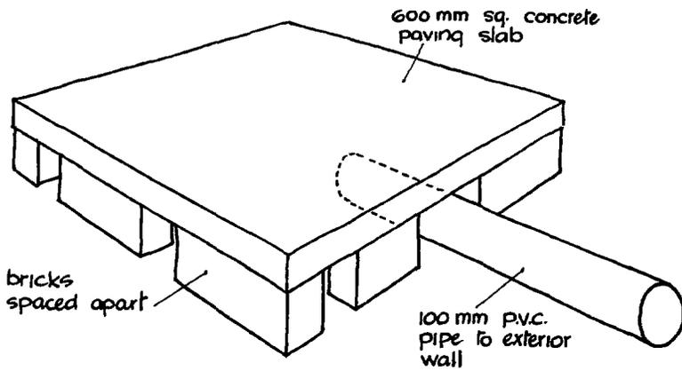
Figure 5: UNDERFLOOR SUMP DETAILS
