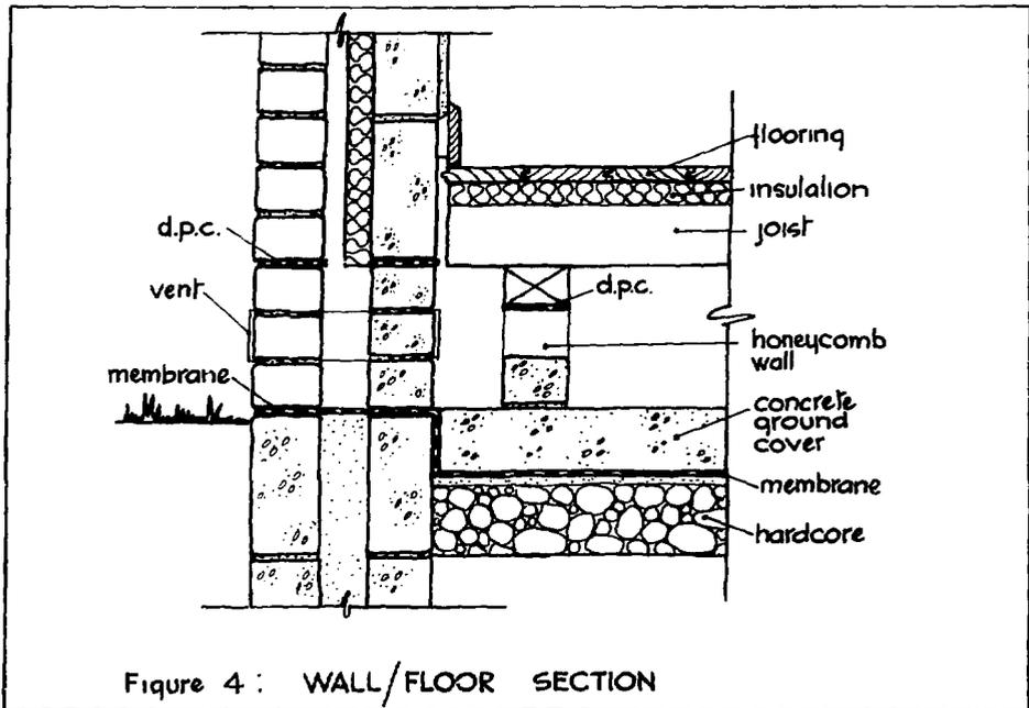
Figure 4 : WALL/FLOOR SECTION
