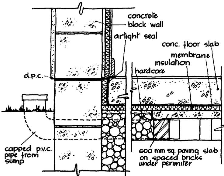
Figure 6: SECTION SHOWING UNDERFLOOR SUMP
