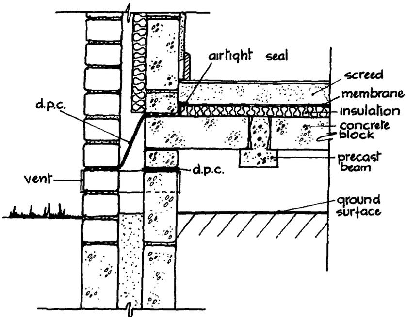
Figure 3: WALL/FLOOR SECTION
