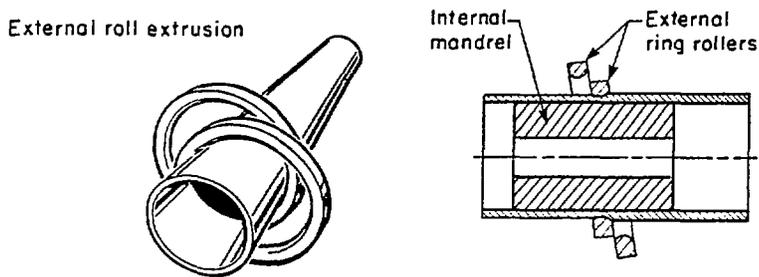
FIGURE 4: Illustration of Process for Cold-Working Cylinders
