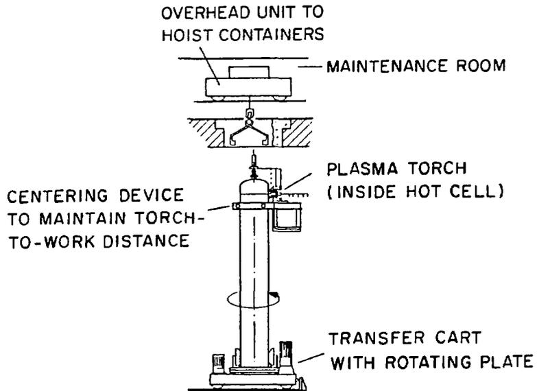
FIGURE 5: Illustration of Plasma-Arc Welding Machine
