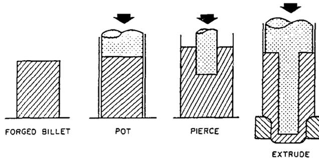
FIGURE 2: Illustration of Closed-End Extrusion Process
