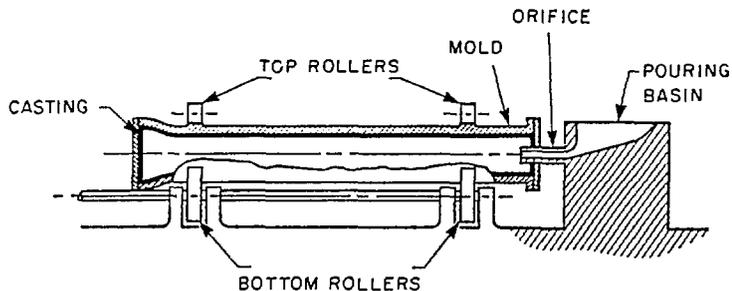
FIGURE 3: Illustration of Centrifugal Casting Machine
