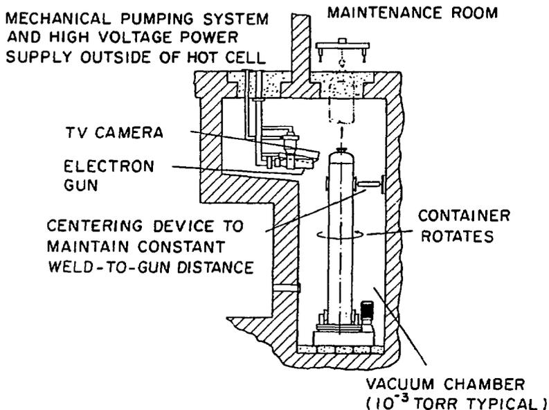
FIGURE 6: Illustration of Electron-Beam Welding Machines
