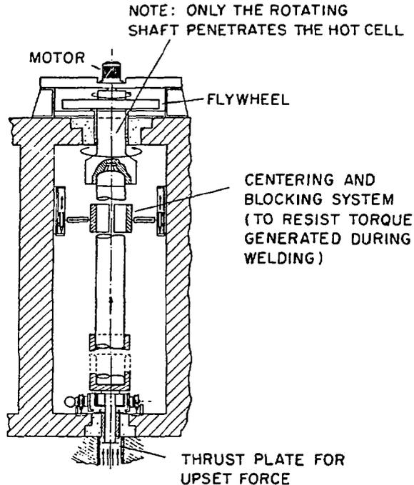
FIGURE 7: Illustration of Friction-Welding Machinery
