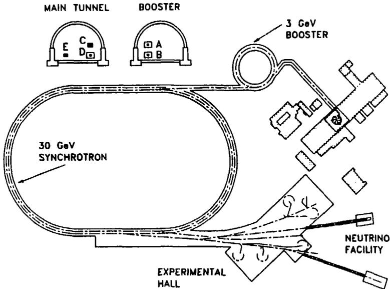
FIGURE 2 Proposed site layout for the TRIUMF KAON Factory.
