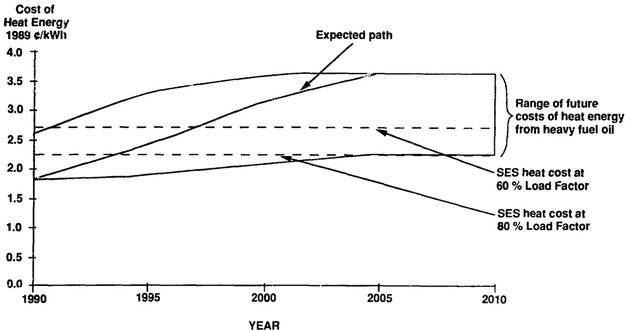
FIGURE 3: COMPARISON OF THE TOTAL COST OF HEAT ENERGY FROM SES WITH THE FUEL COMPONENT COST OF A HEAVY FUEL OIL-FIRED BOILER
