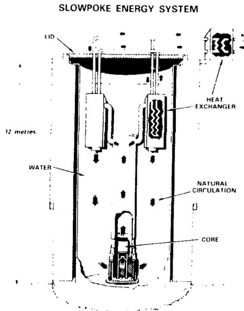
FIGURE 1: SCHEMATIC DIAGRAM OF THE SLOWPOKE HEATING REACTOR CONCEPT
