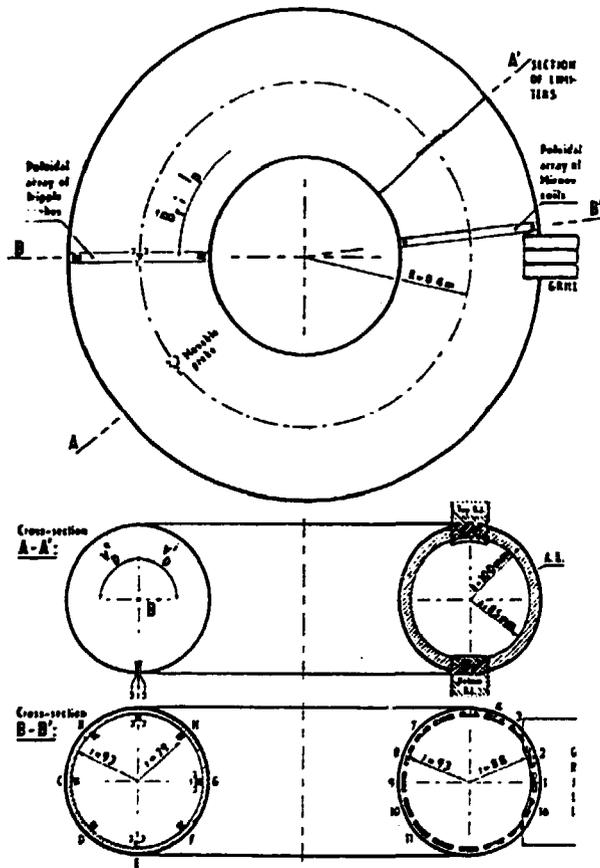
Fig. 11. The geometry of experiment and spacing of diagnostic tools for fluctuation measurements.
