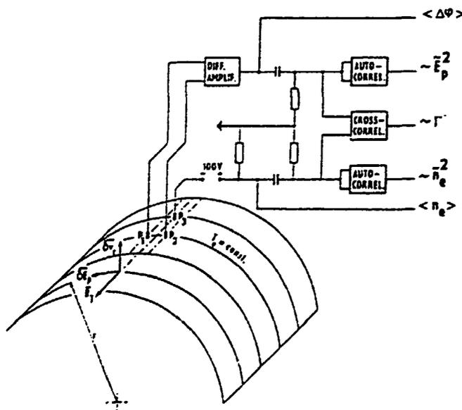
Fig. 12. Schematical arrangement of correlation measurements of the plasma fluctuations.
