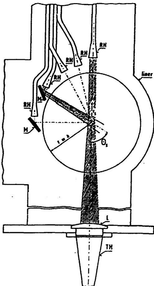
Fig. 13. Geometry of the probing and scattered beams in the small cross-section of tokamak CASTOR.
