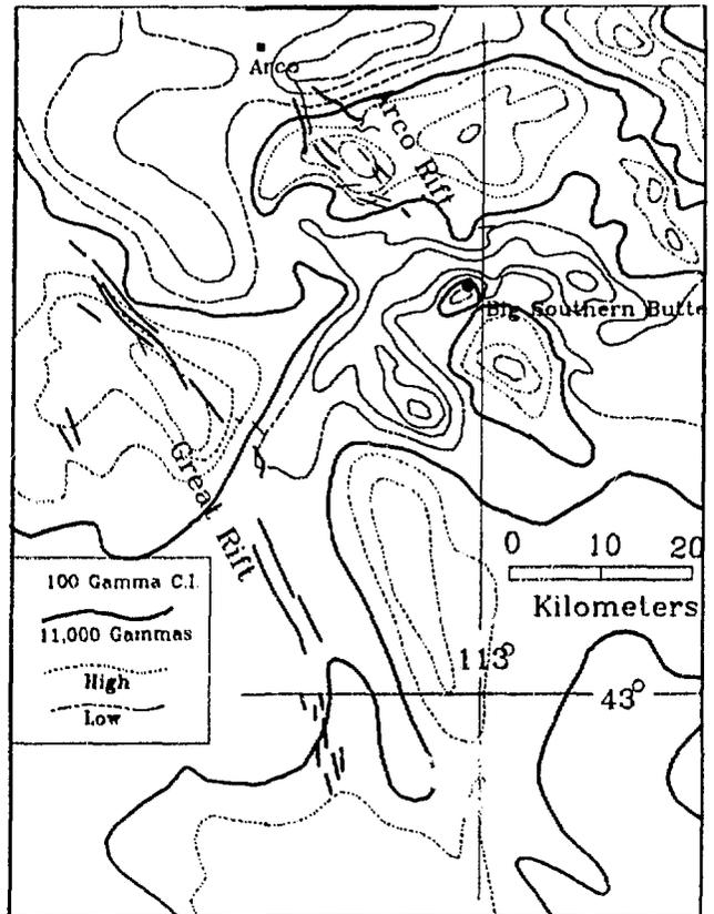
Figure 9. Aeromagnetic anomalies over the Great Rift and the Arco Rift Zone (Modified from Reference [12]).
