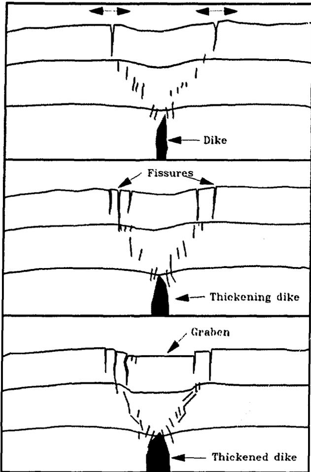
Figure 8. Mastin and Pollard's (1988) idealized depiction of fault and fissure growth above a growing shallow dike (Modified from reference [11]).
