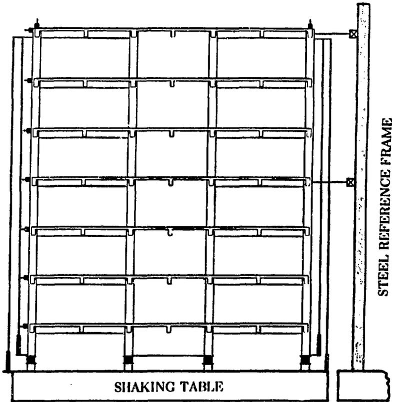
Fig. 4. 1/5-Scale Reinforced Concrete Test Structure
