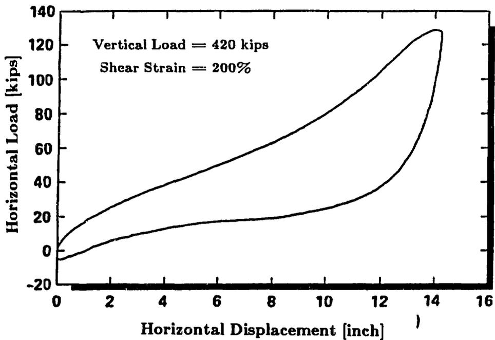
Fig. 3. Shear Force Hysteresis Behavior for Half-Size Seismic Isolator
