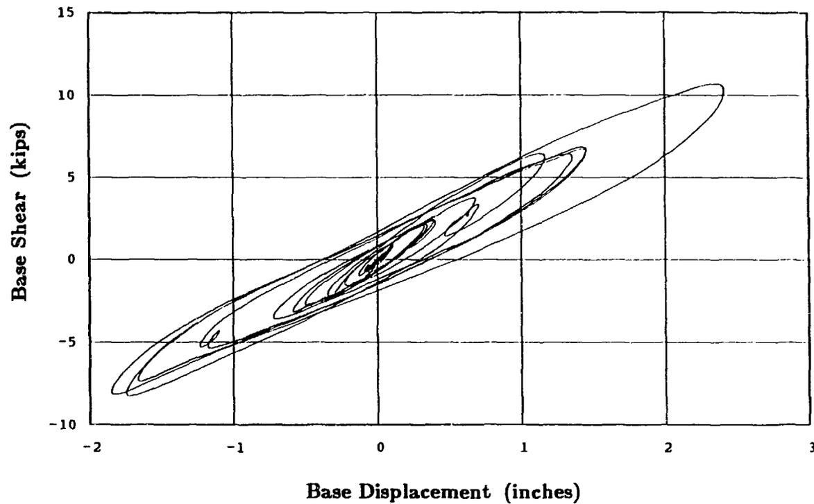
Fig. 9. Shear Hysteresis Behavior of Isolation System.
