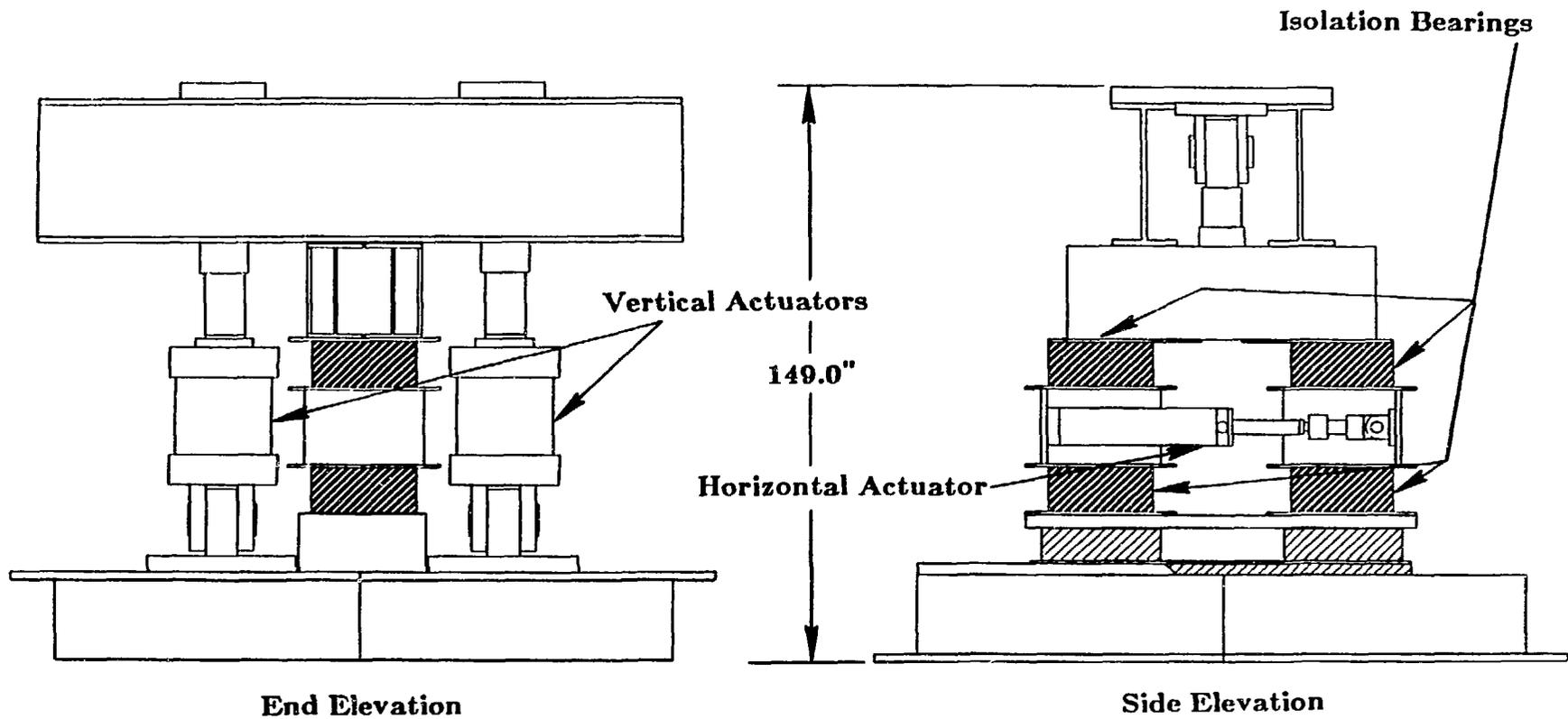
Fig. 2. Large-Scale Bearing Test Rig
