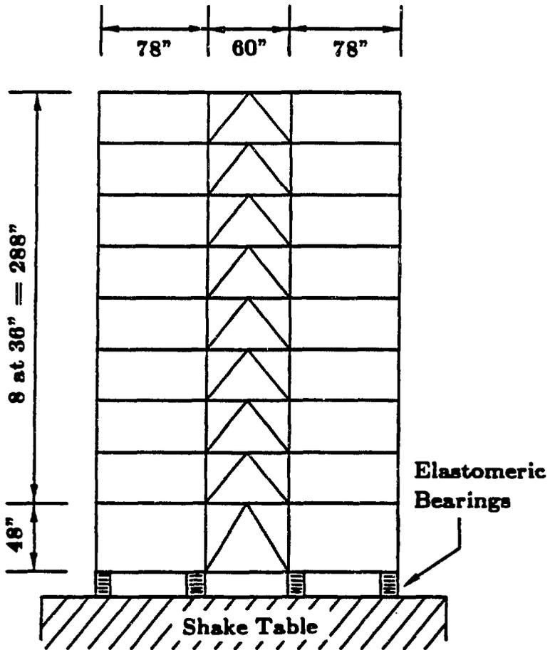
Fig. 5. 1/4-Scale Steel Test Structure
