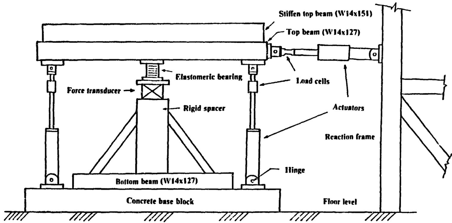
Fig. 1. Single Bearing Shear Test Rig
