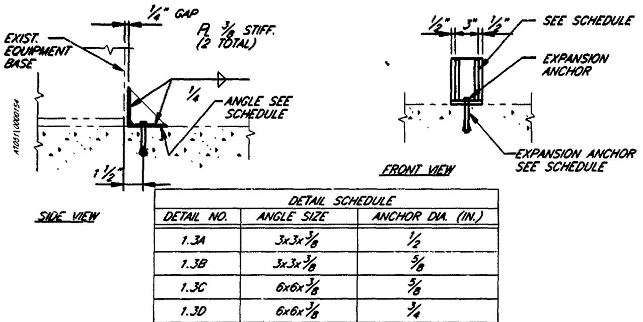
Figure 2. Detail 1.3 - Seismic Stop
