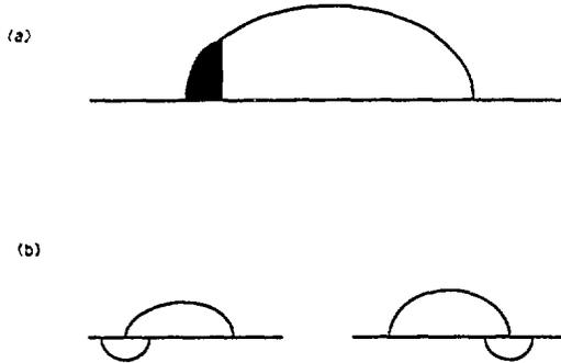
Figure 7: Feynman diagram showing electron self energy. Horizontal line is electron Green's function. Loops are screened electron-electron interaction. Shaded area is vertex correction
