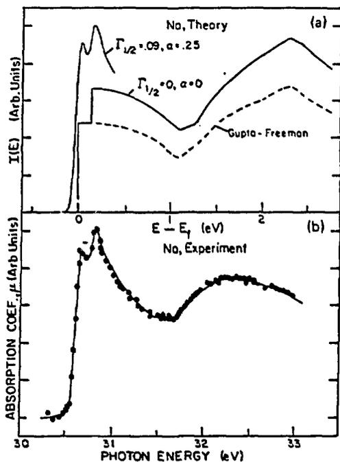
Figure 6: X-ray absorption of metallic sodium. Top shows theoretical prediction, including the two components split by the spin-orbit interaction. Bottom shows experimental data from Callcott et al.<sup>32</sup>
