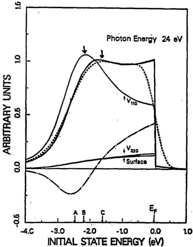
Figure 2: Energy distribution curves for sodium (011) at a photon energy of  $\hbar\omega = 24$  eV calculated by Shung and Mahan<sup>19-20</sup>. The thin solid line shows the interband contribution alone. Its peak denotes the interband transition. The heavy solid line combines the surface and volume effects. The peak position is 0.2-0.3 eV higher, because of surface effects. Identifying this as the interband point would lead to apparent narrowing, which is in fact only interference.
