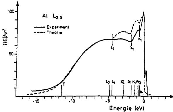
Figure 5: L emission spectra of metallic aluminum, from Neddermeyer<sup>24</sup>.
