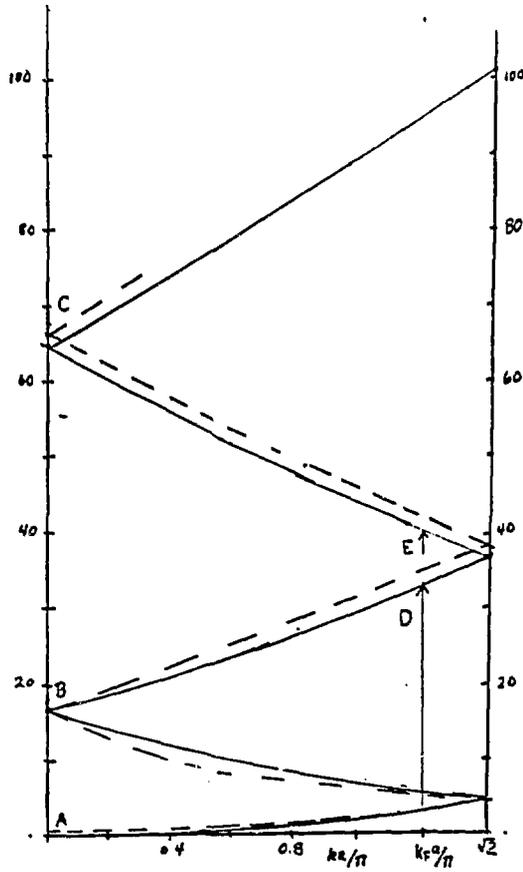
Figure 4: Energy bands in Na projected in the (011) direction. The solid lines are free electron bands, while the dashed line are the bands including the screened exchange energy.
