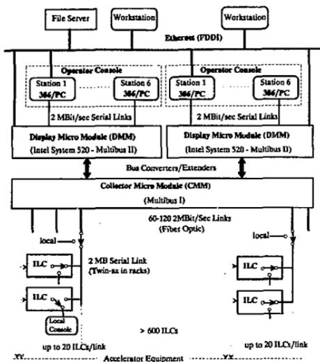
Fig. 3. The highly distributed architecture of the ALS computerized control system.
