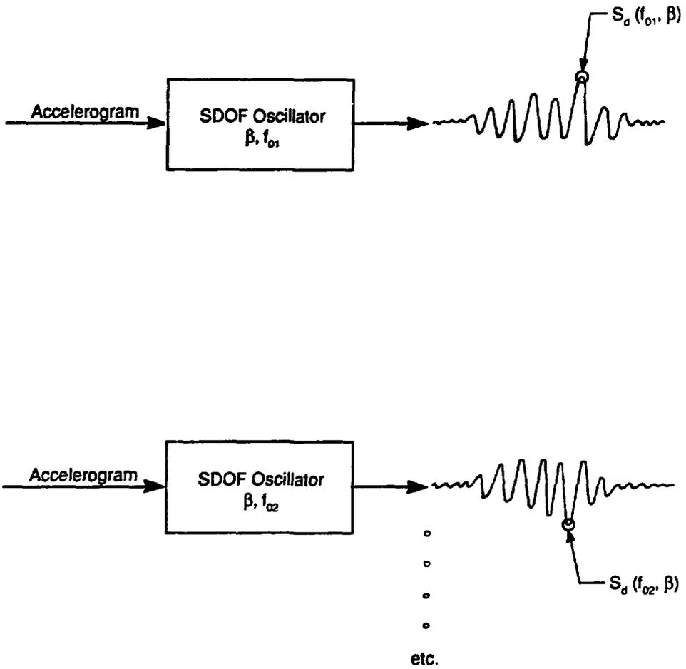
A plot of  $S_d$  versus frequency is the displacement response spectrum.
