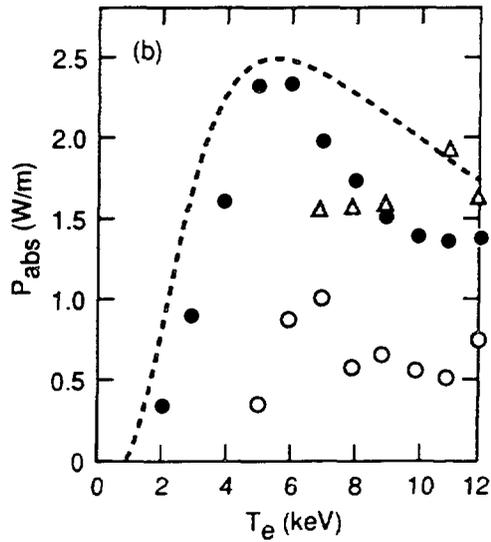
Fig. 3. (a) Current drive efficiency  $\gamma$  and (b) power absorption vs electron temperature for three scenarios in DIII-D: (1)  $k_{\perp} \sim 7 \text{ m}^{-1}$  and  $f = 60 \text{ MHz}$  (solid circles); (2)  $k_{\perp} \sim 7 \text{ m}^{-1}$  and  $f = 120 \text{ MHz}$  (open circles); and (3)  $k_{\perp} \sim 5 \text{ m}^{-1}$  and  $f = 60 \text{ MHz}$  (open triangles).
