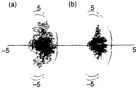
Fig. 1. Contours of electron power absorption in ITER (a) including  $k_{\parallel}$  variations and (b) with  $k_{\parallel} = k_{\perp}$ .
