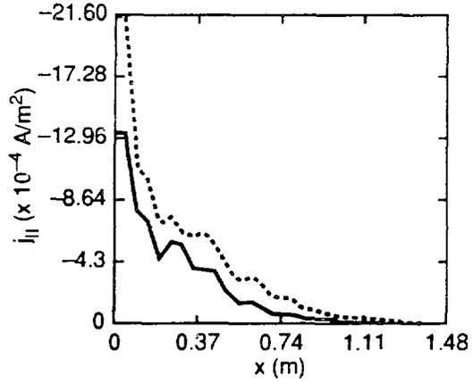
Fig. 2. Flux surface average of the driven current density in ITER with  $k_{\parallel}$  variations included (solid) and with  $k_{\parallel} \sim k_{\perp}$  (dashed).
