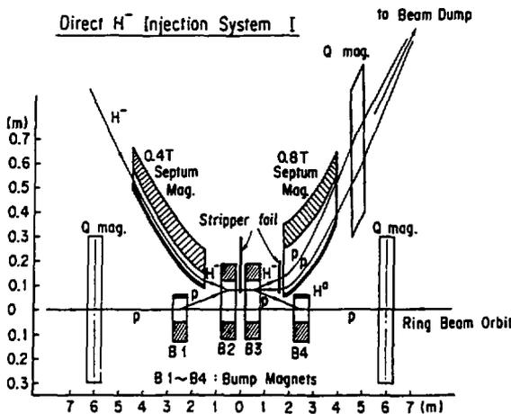
Fig. 5 Direct  $H^-$  injection system I.
