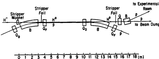
Fig. 7 Example of a two-step  $H^0$  injection system.
