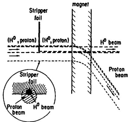
Fig. 4 Beams upstream and downstream of the stripper foil during  $H^0$  injection.
