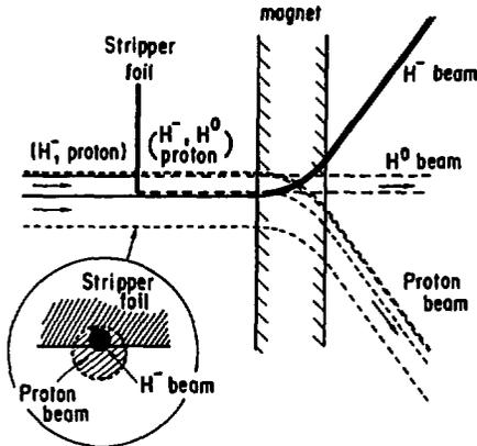
Fig. 3 Beams upstream and downstream of the stripper foil during  $H^-$  injection.
