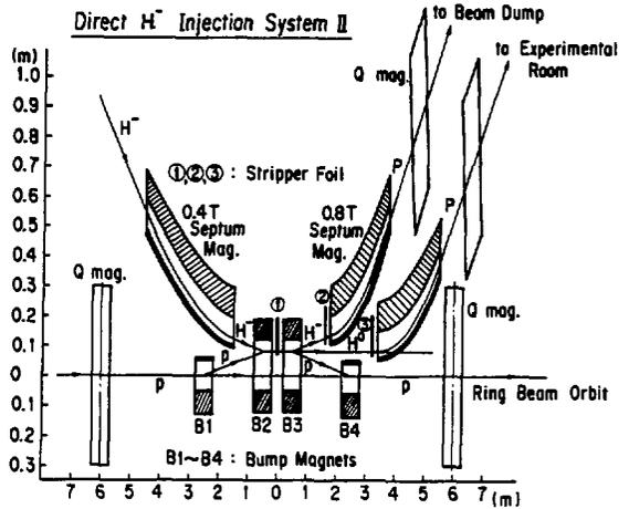
Fig. 6 Direct  $H^-$  injection system II.
