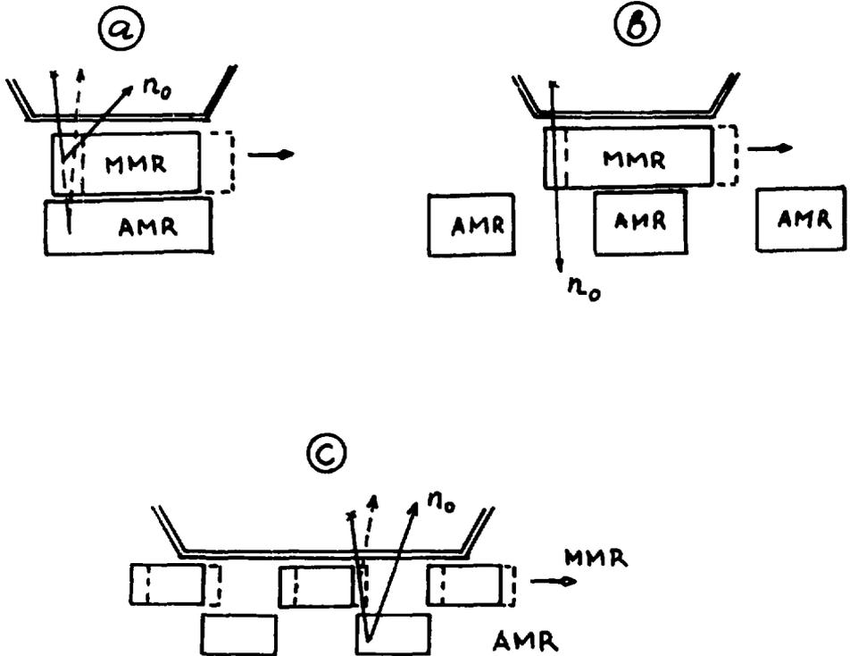
Fig.4 The diagrams of moving reflectors geometry to explain the "shadow" effect of neutron reflection. a-the first version of MR; b- MR-2; c-MR-3.
