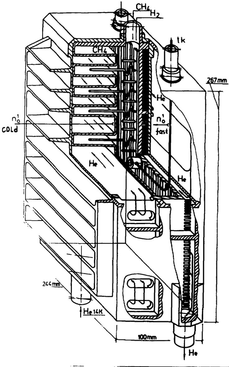
Fig.6. The solid methane moderator of IBR-2, the cross-section drawing of the methane and helium cameras.
