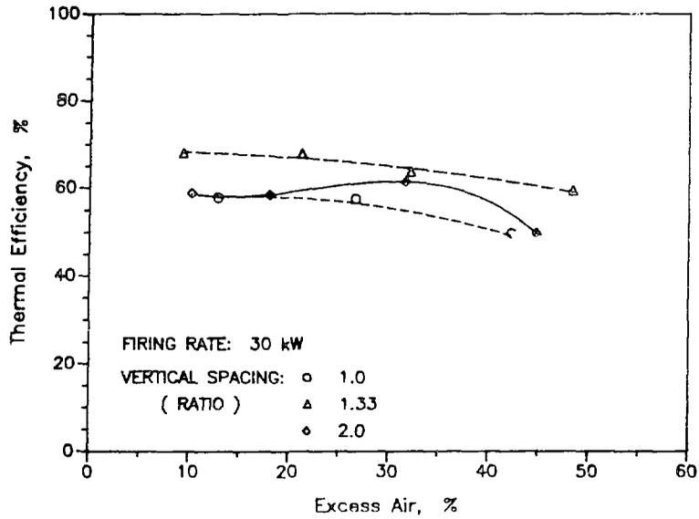
Figure 8. EFFECT OF VERTICAL SPACING OF TUBES ON THERMAL EFFICIENCY
