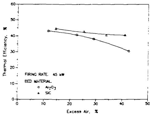
Figure 13. EFFECT OF BED MATERIAL ON THERMAL EFFICIENCY
