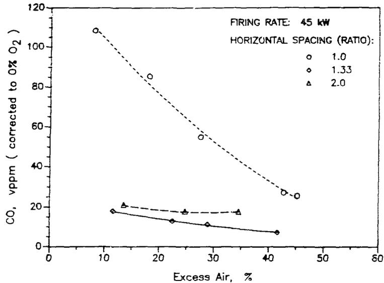
Figure 12. EFFECT OF HORIZONTAL SPACING OF TUBES ON CO EMISSIONS
