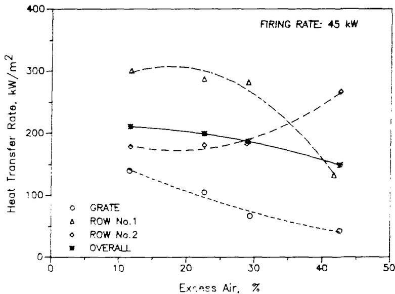
Figure 3. EFFECT OF EXCESS AIR ON HEAT-TRANSFER RATES
