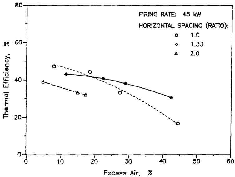
Figure 11. EFFECT OF HORIZONTAL SPACING OF TUBES ON THERMAL EFFICIENCY
