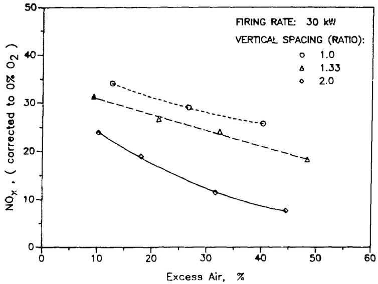
Figure 9. EFFECT OF VERTICAL SPACING OF TUBES ON NO<sub>x</sub> EMISSIONS
