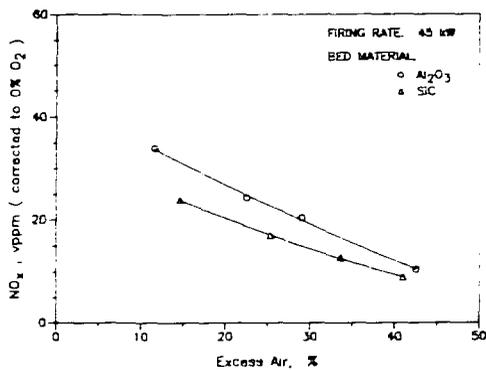
Figure 14. EFFECT OF BED MATERIAL ON NO<sub>x</sub> EMISSIONS
