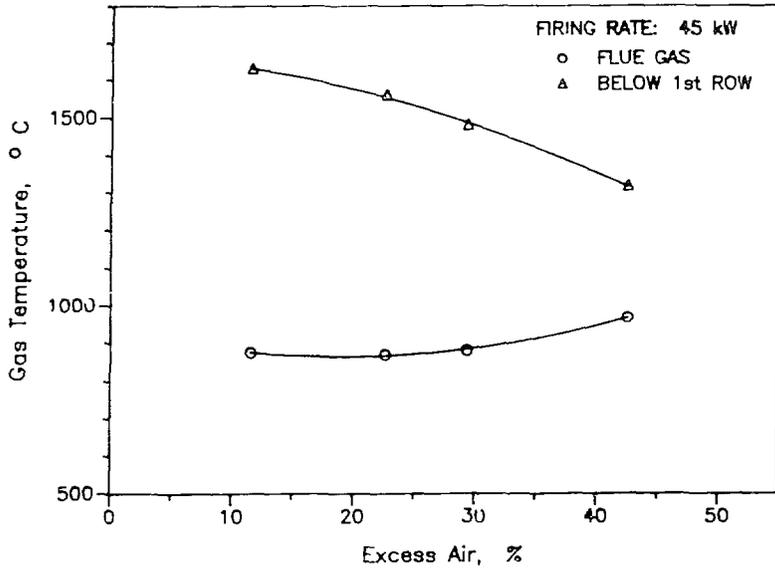
Figure 4. EFFECT OF EXCESS AIR ON GAS TEMPERATURE
