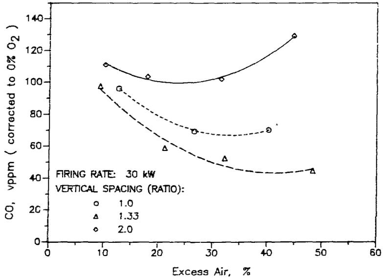
Figure 10. EFFECT OF VERTICAL SPACING OF TUBES ON CO EMISSIONS
