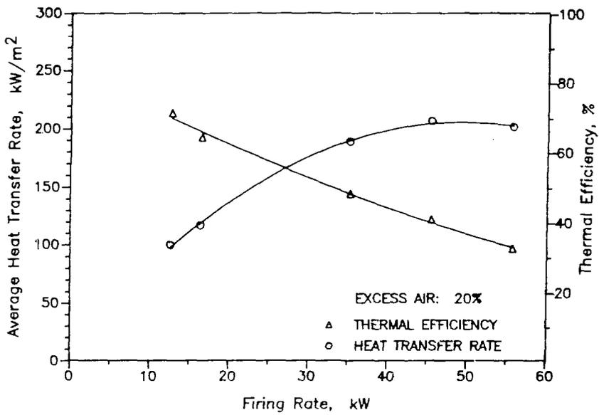
Figure 7. EFFECT OF FIRING RATE ON OVERALL HEAT TRANSFER
