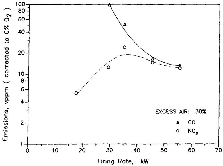
Figure 6. EFFECT OF FIRING RATE ON COMBUSTION EMISSIONS
