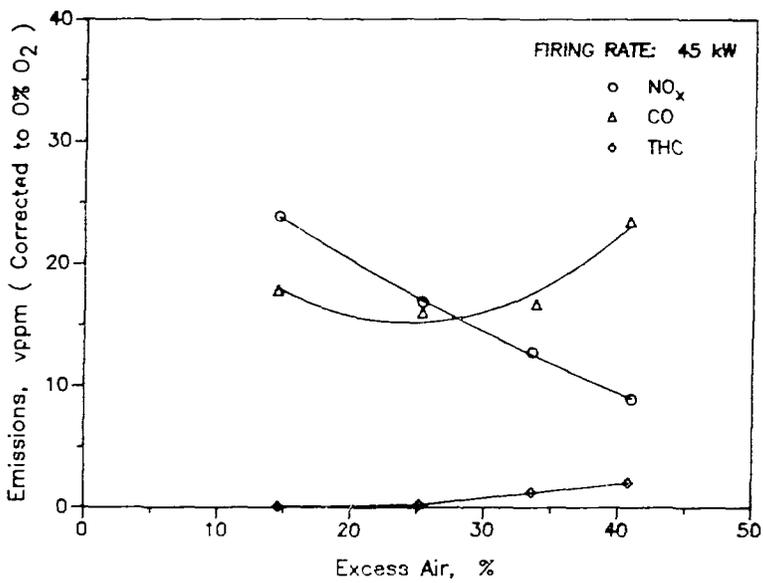
Figure 5. EFFECT OF EXCESS AIR ON COMBUSTION EMISSIONS
