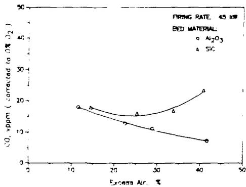
Figure 15. EFFECT OF BED MATERIAL ON CO EMISSIONS
