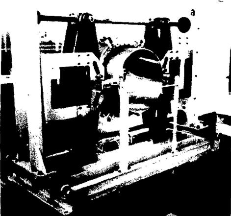
Fig. 5. Vacuum flange disconnect system.
