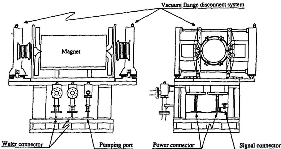
Fig.3. The magnet assembly with quick-disconnect devices.
