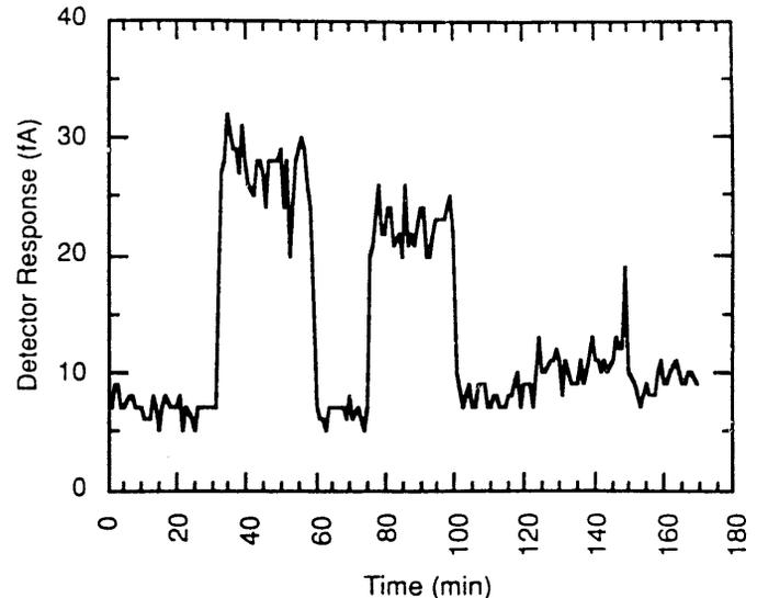
Fig. 7. Response of the LRAD system to a contaminated block (35-60 min); a 200-dpm  $^{239}\text{Pu}$  source (75-100 min); and a relatively uncontaminated block (125-150 min). Removing the block caused the spike at 150 min. All regions between the measurements represent detector background.
