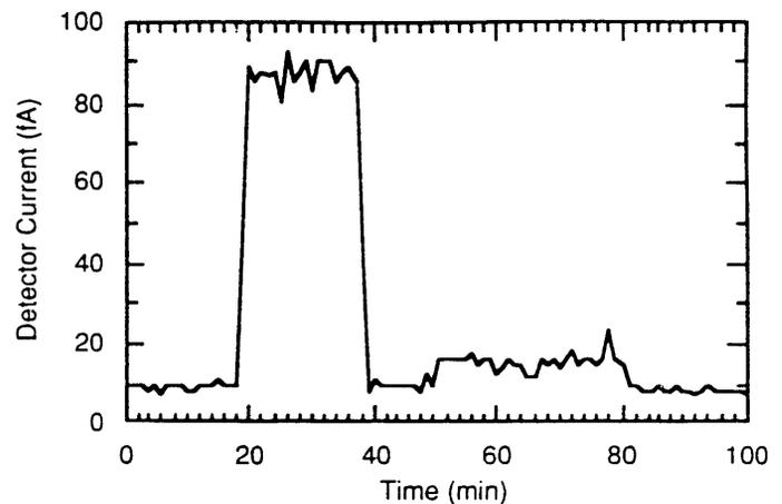
Fig. 4. Response (from left to right) of the LRAD to 1000-dpm and 100-dpm  $^{239}\text{Pu}$  alpha sources. The detector response is averaged in one-minute intervals.
