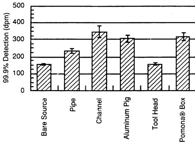
Fig. 6. Minimum detectable source strengths (with 99.9% certainty) in each of the five mockups illustrated in Fig. 5, as well as the minimum detectable bare source.
