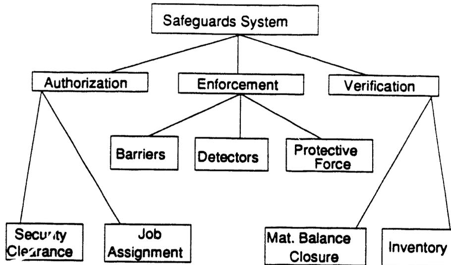
**Fig. 3. Decomposition of an integrated safeguards system into subcomponents.**
