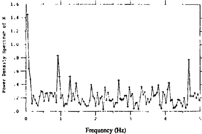
**Figure 40** The Fourier transform of the data in Figure 39 showing white noise with additional power near 0 and 1 Hz.
