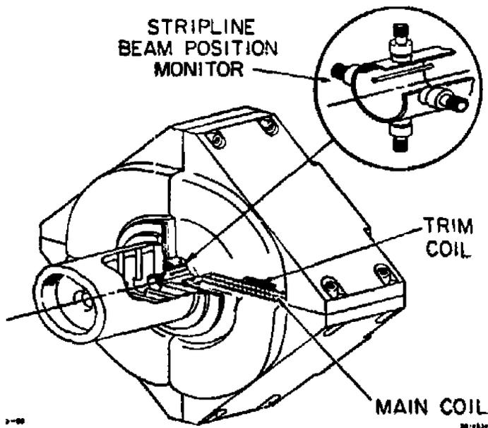
Figure 2 Schematic view of a strip line beam position monitor.
