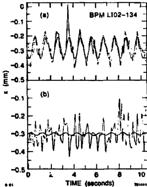
Figure 41 Measured bunch position as a function of time (straight lines) for two periods separated by 3 minutes. The sine curve is a fit to the data at 1.2 Hz. Note that the frequency spectrum of the beam jitter can change rapidly, even though the root-mean-square jitter is about the same.
