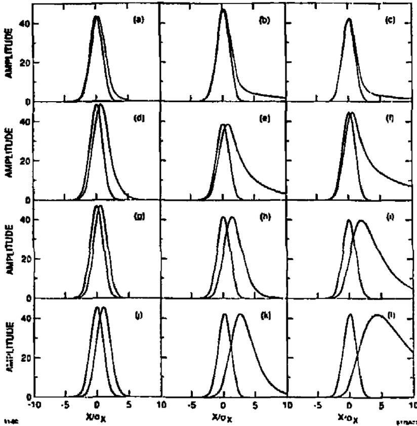
Figure 38 Calculated transverse bunch projections showing the effects of different input conditions with the rate of tail growth  $\tau$  and the place  $z_0$  along the bunch where the exponential growth starts. Large  $\tau$  (horizontal axis) makes long thin tails and a  $z_0$  closer to the front of the bunch (vertical axis) makes a broader shoulder.
