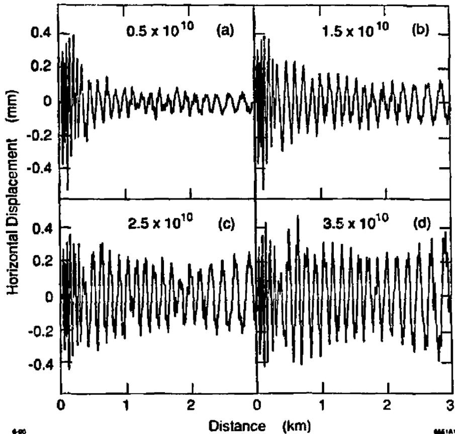
Figure 20a Observed driven single bunch oscillations along the linac versus charge. Standard BNS conditions for  $3 \times 10^{10} e^-$  are used in all cases but with the linac overall phase adjusted to make a small energy spectrum at 47 GeV. Note that at high charge, damping from acceleration is not as strong as wakefield growth in the latter half of the linac.
