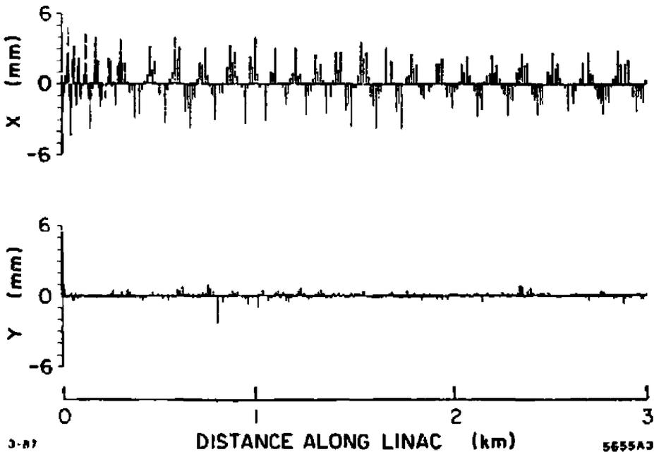
Figure 3 Observed betatron oscillation in the SLC linac induced by a horizontal dipole change near the beginning. From small quadrupole roll errors, a small oscillation is coupled in, then out, of the vertical plane in the region 600 to 1200 m.
