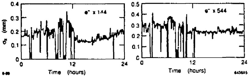
Figure 44 Measured bunch sizes as a function of time for two profile monitors located 90 degrees apart in betatron phase (47 GeV). Both the emittance and the betatron function of the beam are changing with time. Note that the time over which these beam parameters change is quite long.
