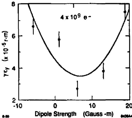
Figure 17 Dispersion increased emittance at 47 GeV with an oscillation starting early in the linac. The low bunch charge makes very small wakefield effects.
