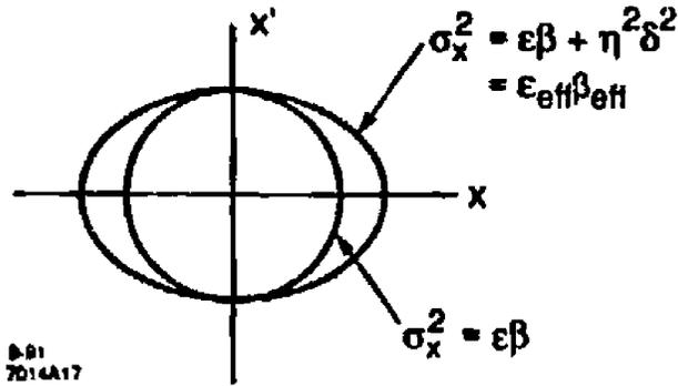
**Figure 32** A dispersion mismatch  $\eta$  ( $\eta'$ ) combined with an energy spread  $\delta$  produces an new effective emittance and  $\beta$  ( $\alpha$ ) of the beam. Standard emittance measurements obtain these effective parameters.
