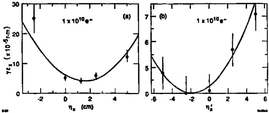
**Figure 33** Emittance measurements at the end of the SLC accelerator as a function of dispersion errors at injection. The solid lines are theoretical predictions.
