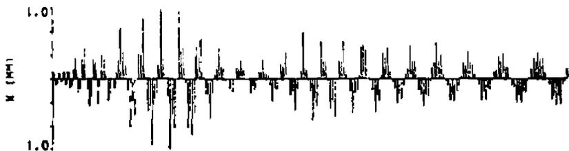
Figure 20b Observed oscillation for a single bunch when the energy spectrum is not properly set along the linac. Apparent trajectory beating can be seen.
