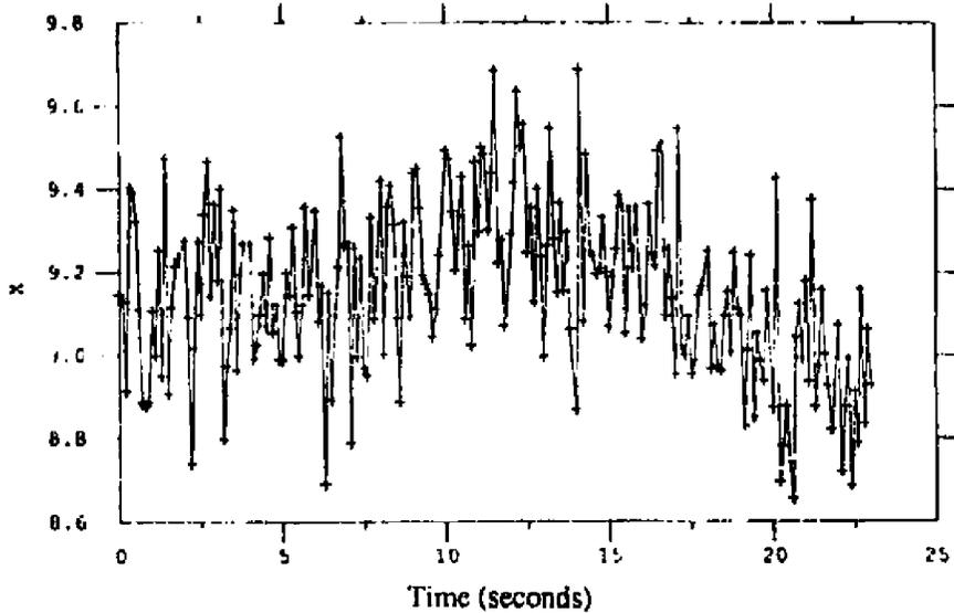
**Figure 39** Measured beam position (mm) at one location (monitor) on every accelerator pulse as a function of time. Straight lines connect the data. Note the fast and slow drifts. A single position measurement has an error of about 20 microns.
