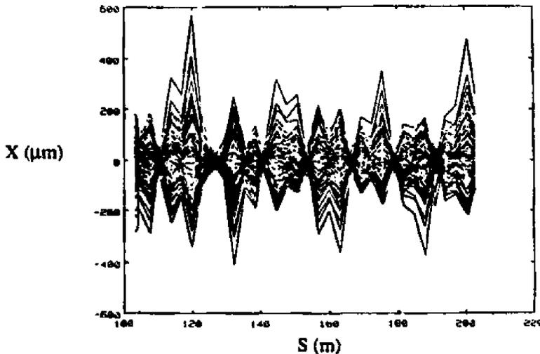
Figure 42 Measured single-pulse beam trajectories superimposed for multiple pulses. The amplitude of the position jitter changes with time but the phase of the oscillation is always the same. If the monitoring system is available, this envelope plot can be traced back to the jitter source. The relative position measurement errors from monitor to monitor can also be studied with this data.
