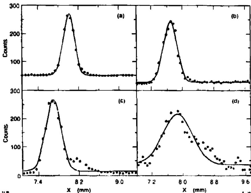
Figure 37b Measured beam profiles (47 GeV) for the betatron oscillation in Figure 37a. The projections were taken with four wire scanners spaced at (a) 0, (b) 22.5, (c) 90., and (d) 112.5 degrees in betatron phase. Note that the induced transverse tail has a particular phase such that the tail does not appear at position (a). The produced profiles have different shapes depending on the betatron phase. Consequently, the transverse tail rotates in phase space at the betatron frequency.
