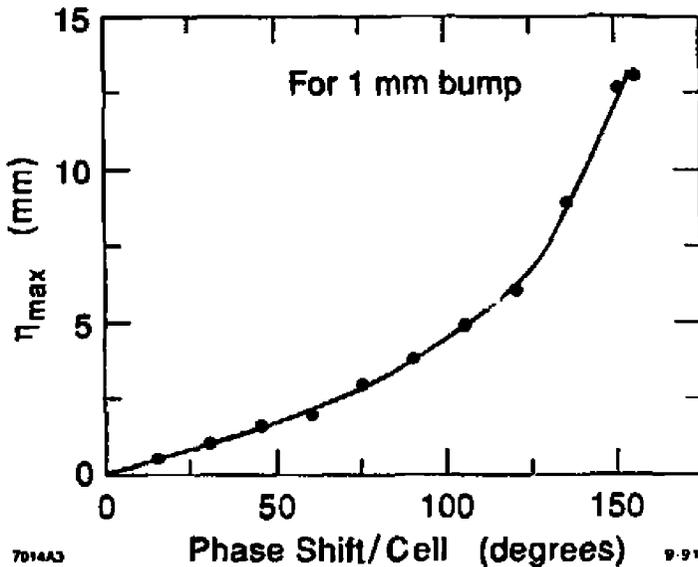
Figure 15b The dispersion generated from a single beam bump as a function of phase advance per cell. The dispersion increases nonlinearity with lattice strength. The bump is closed for all energies with the quadrupoles off.
