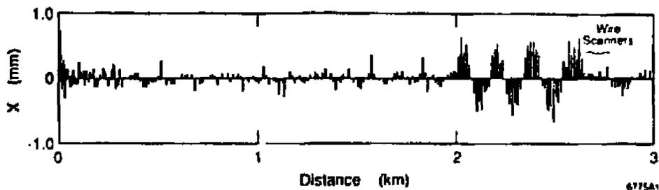
Figure 37a Induced horizontal oscillation of an SLC electron bunch which generates transverse tails from wakefields.  $\sigma_z = 1. \text{ mm}$  and  $I = 3. \times 10^{10} \text{ e}^-$ .
