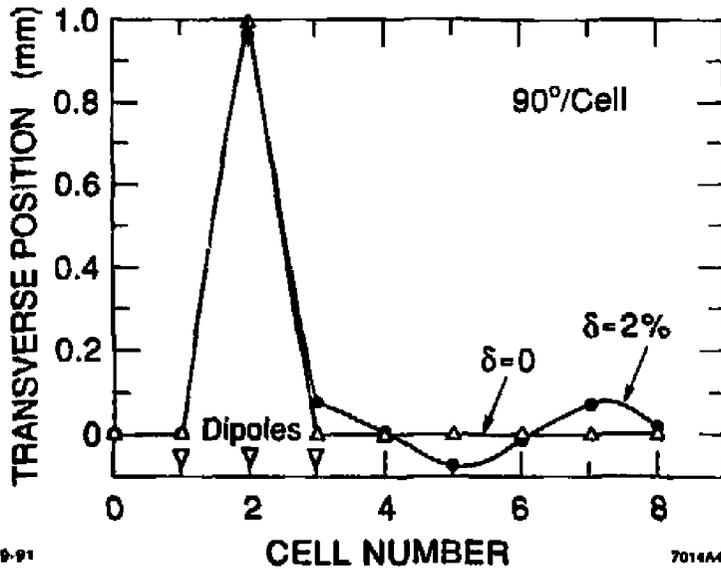
Figure 15a Dispersion is generated from a closed dipole beam bump in a quadrupole lattice. There are two quadrupoles per cell. If the bump is closed for an on-energy particle ( $\delta = 0$ ), then the bump is not closed for off energy particles. Trajectory correction, in general, can be viewed as a series of beam bumps.
