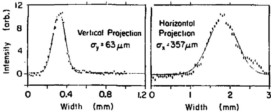
Figure 26 Typical measurements of vertical and horizontal beam sizes. A Gaussian fit has been performed on the data. Non-Gaussian beam shapes can affect the fitting process. Screen profile monitors can measure a beam shape on a single accelerator pulse. Wire scanners require many pulses or many wires.
