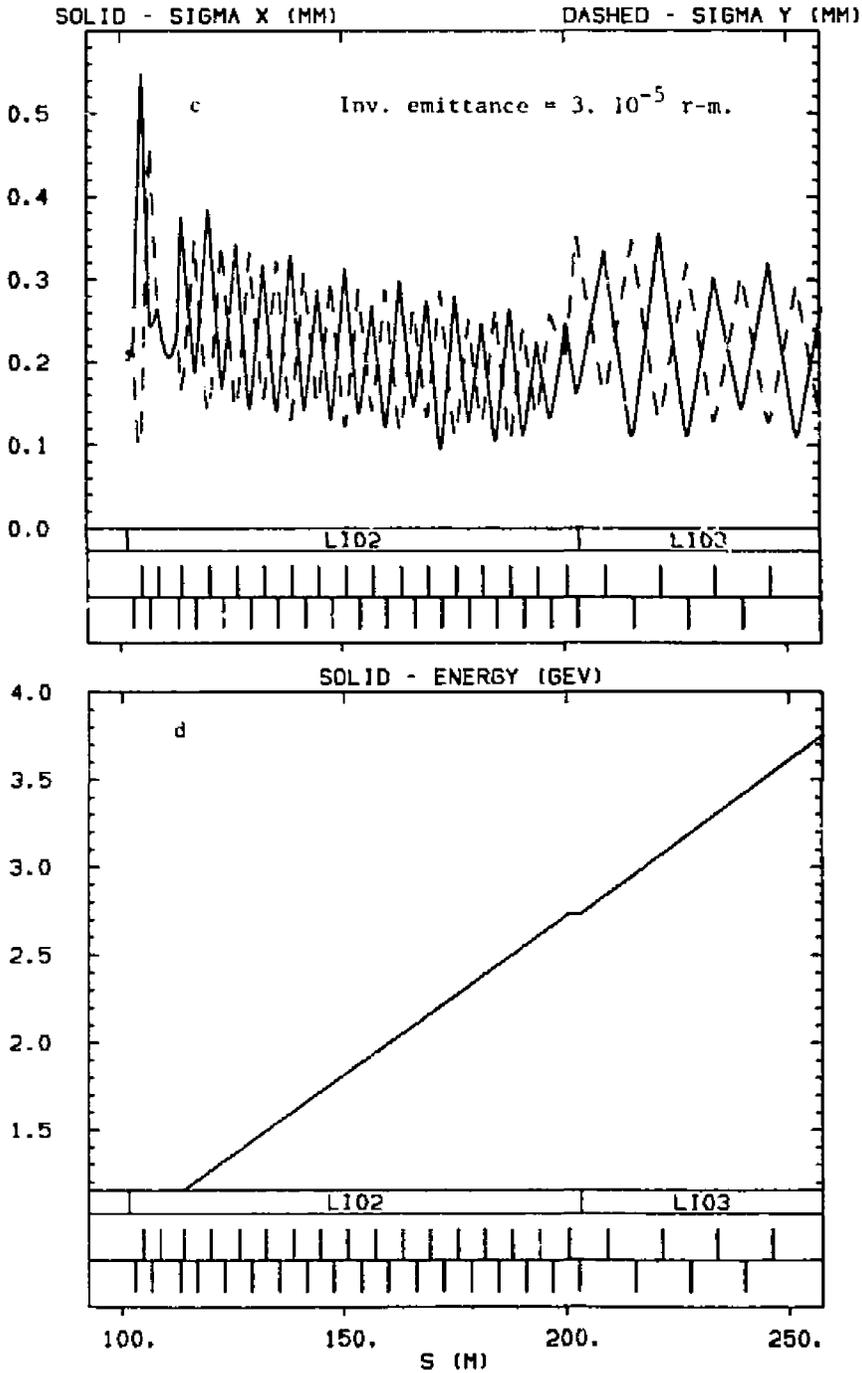
Figure 4c,4d Plots of the beam sizes and energy profile over the first 150 m.
