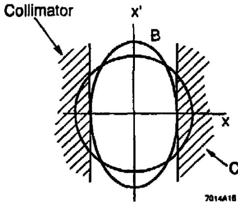
Figure 30 A collimator which cuts the position edges of a beam makes the beam have a new effective  $\beta$  and  $\alpha$ , until filamentation restores them. The emittance of the beam is reduced until filamentation also restores it.
