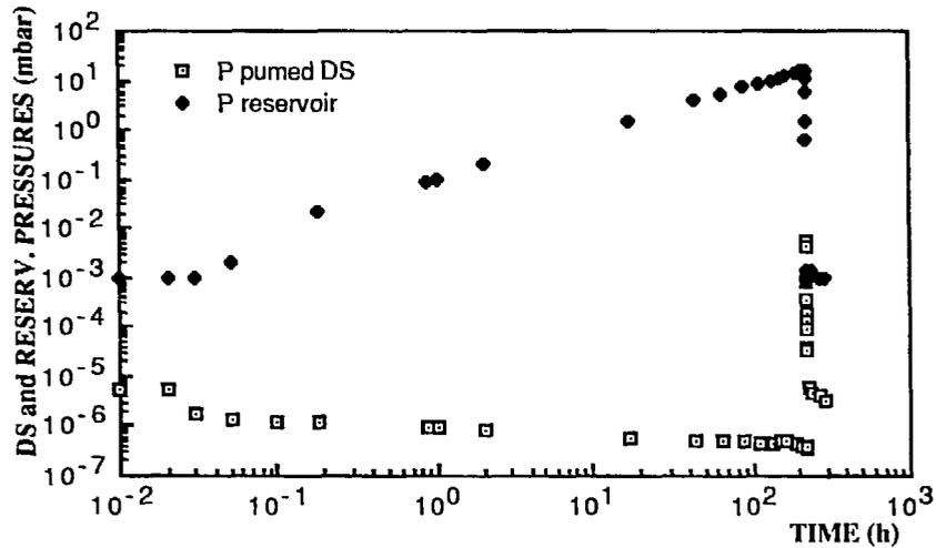
Fig. 3 Dead section and reservoir pressures during the second and third step of the turbomolecular pumping test.
