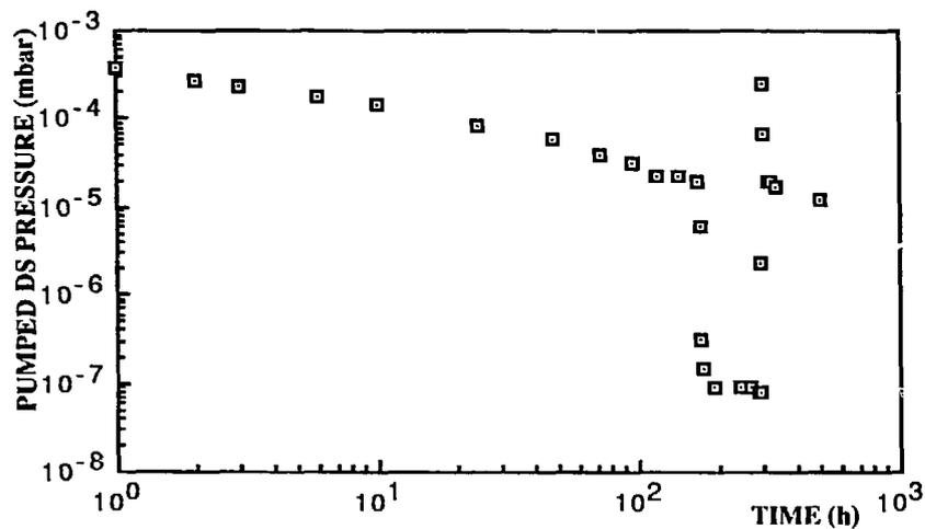
Fig. 5 Dead section pressure during the cryogenic pumping test.
