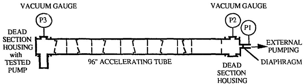
Fig. 1 Experimental equipment used for the dead section pump tests.
