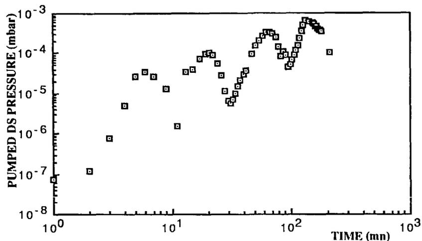
Fig. 6 Dead section pressure during the outgasing step of the cryogenic pump.
