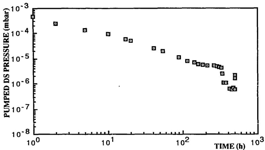
Fig. 4 Dead section pressure during the ion getter pumping test.
