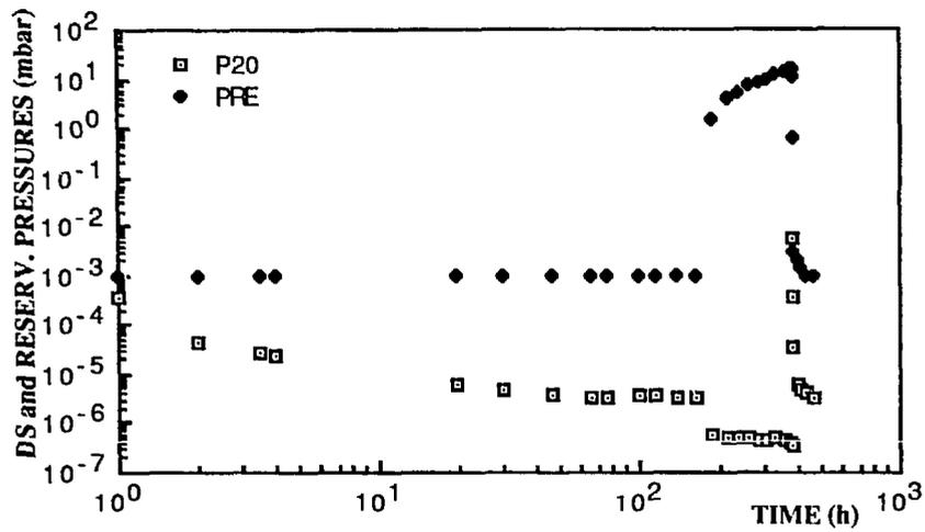
Fig. 2 Pressures during the three steps of the turbomolecular pumping test.
