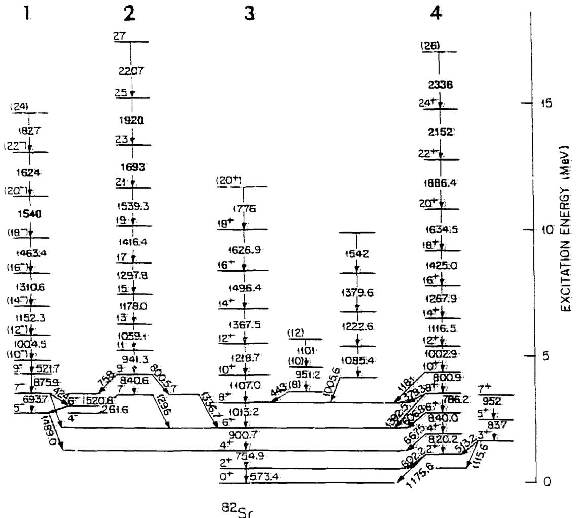
Fig. 4 Partial level scheme for  $^{82}\text{Sr}$  showing four major rotational bands. Band 3 is the ground band, and band 4 is the yrast one. The odd spin band 2 becomes yrast at spins higher than 23.
