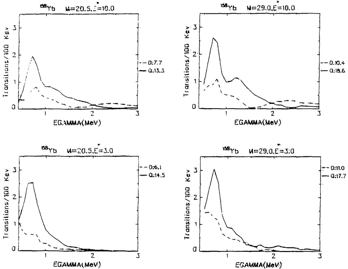
Fig. 2 Evolution of the quadrupole (solid lines) and dipole (dashed lines) spectra with excitation energy ( $E^*$ ) and multiplicity ( $M$ ). Each panel is labeled with the corresponding values of  $E^*$  and  $M$ . Noteworthy structures that become strong at high multiplicities are: A quadrupole bump ( $E_\gamma \approx 1.15$  MeV); and a broad dipole structure ( $E_\gamma \approx 1.5-3$  MeV) at high  $E^*$ ; and a low-energy continuum dipole at low  $E^*$ .
