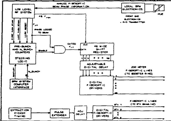
Fig. 4 Block Diagram of Sequencer.
