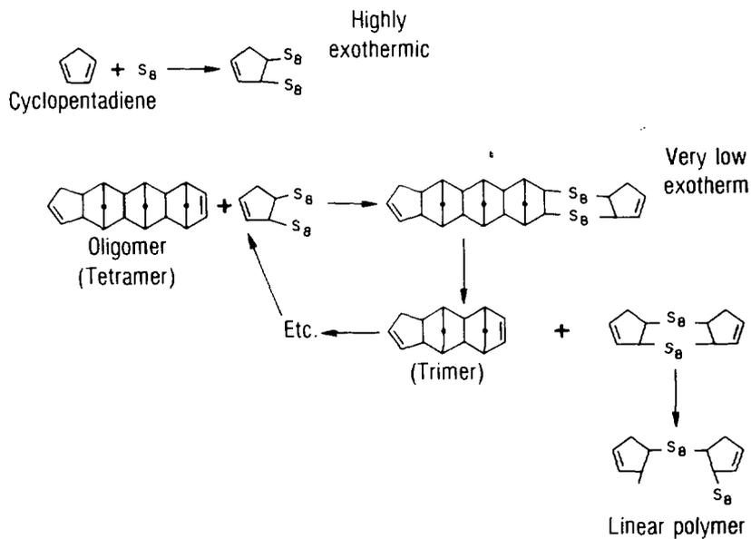
Figure 1. Generalized reaction for sulfur cement production employing mixed modifier
