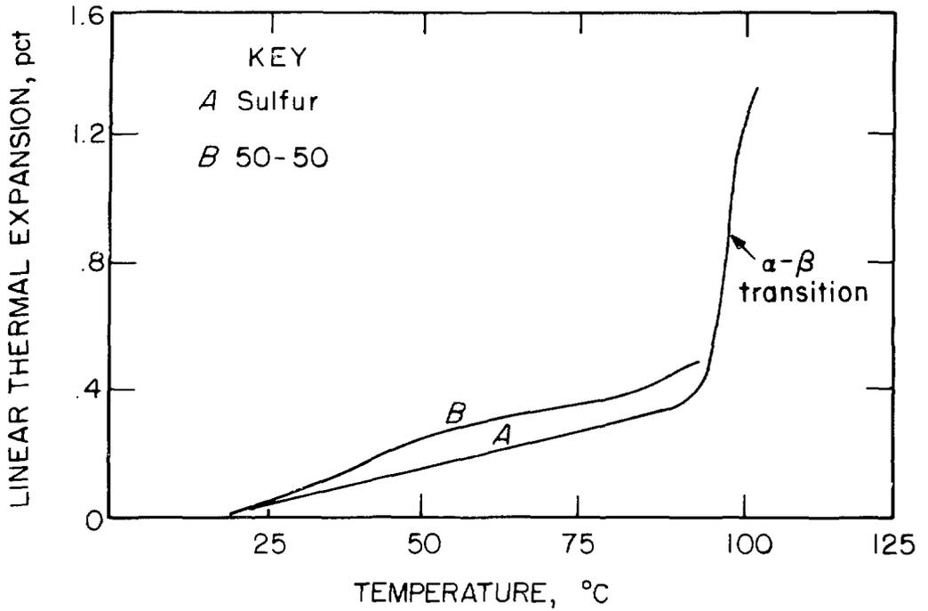
Figure 3. Linear thermal-expansion data for sulfur and sulfur concrete
