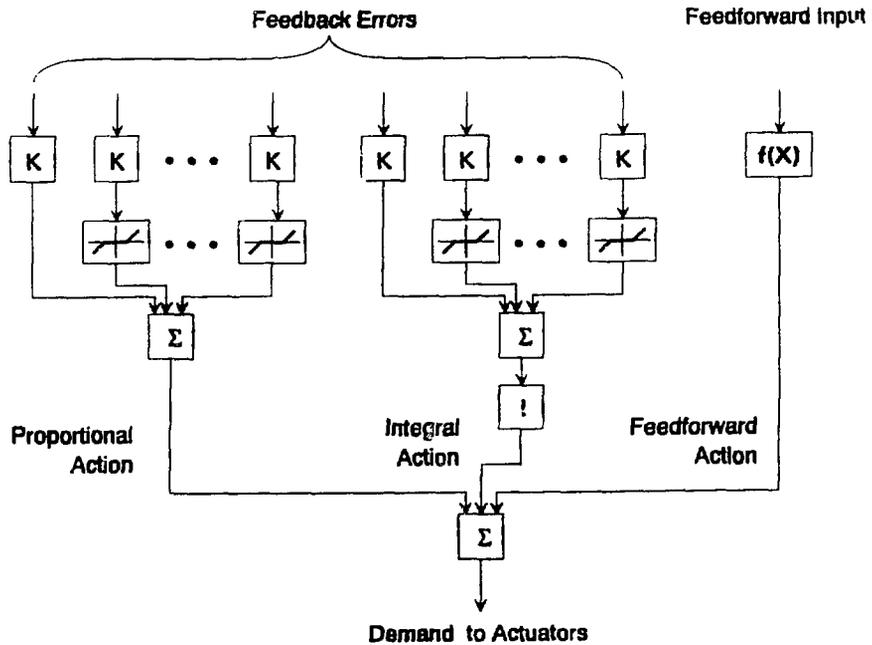
Figure 1. General arrangement of the multivariate controller.
