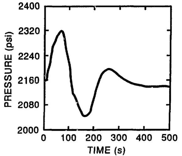
Figure 4. The feedwater pump trip transient demonstrates response to a disturbance that momentarily exceeds the capacity of the actuators.
