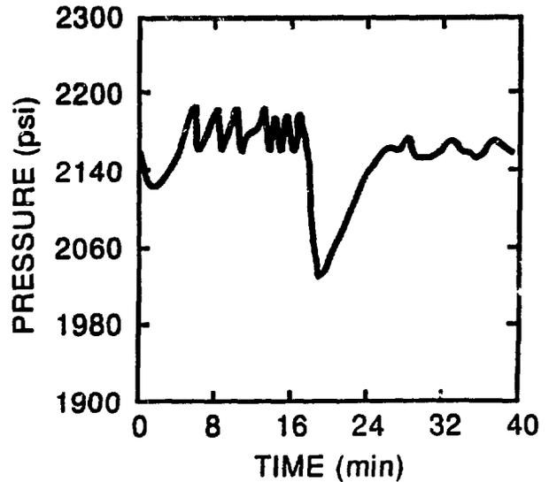
Figure 3. The normal power ramp demonstrates performance of the control system in fully automatic mode.
