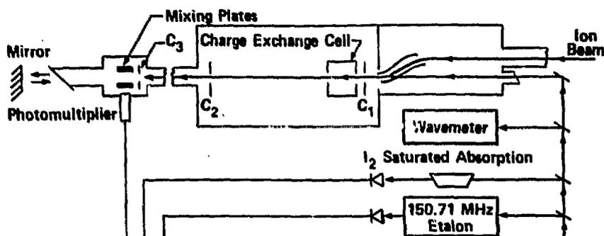
Figure 4. Schematic of the interaction region of the UNISOR laser facility when configured to measure resonating wavenumbers for parallel or antiparallel beams.
