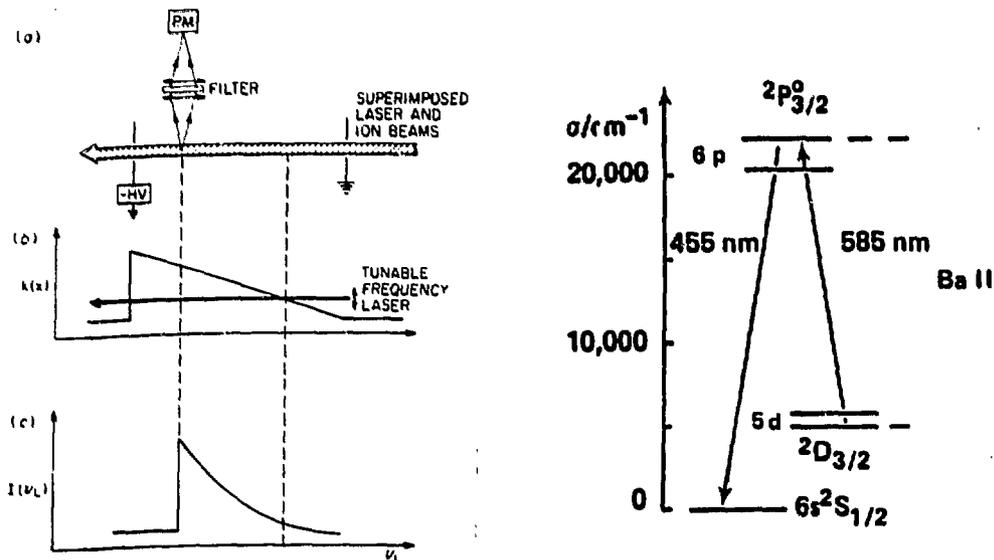
Figure 2. Principle of the rapid Doppler switching method. (a) Schematic of the experimental arrangement showing the collinear beams passing through a parallel plate capacitor. (b) The ion kinetic energy as a function of position along the common beam axis. (c) The expected variation of the recorded fluorescence as a function of laser frequency. (d) Partial energy level diagram of Ba II showing the transitions used in the present investigation.
