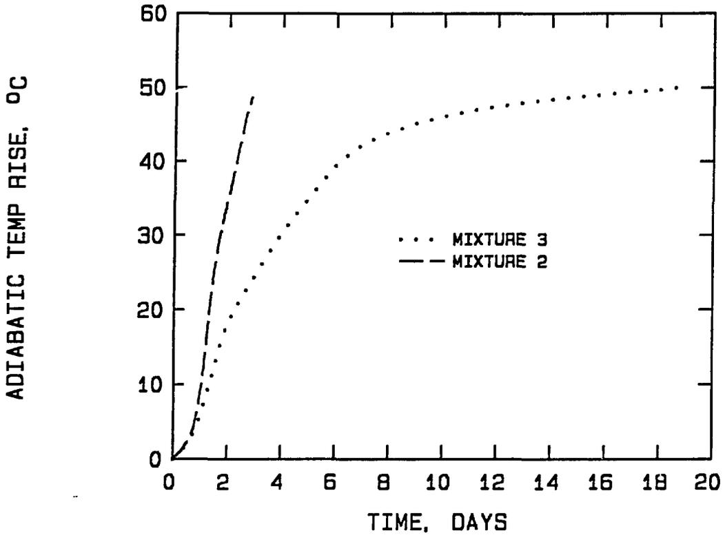
FIGURE 5. HANFORD COLD CAP ADIABATIC TEMPERATURE RISE
