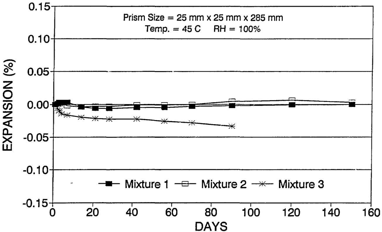
FIGURE 2. HANFORD COLD CAP VOLUME STABILITY VS TIME
