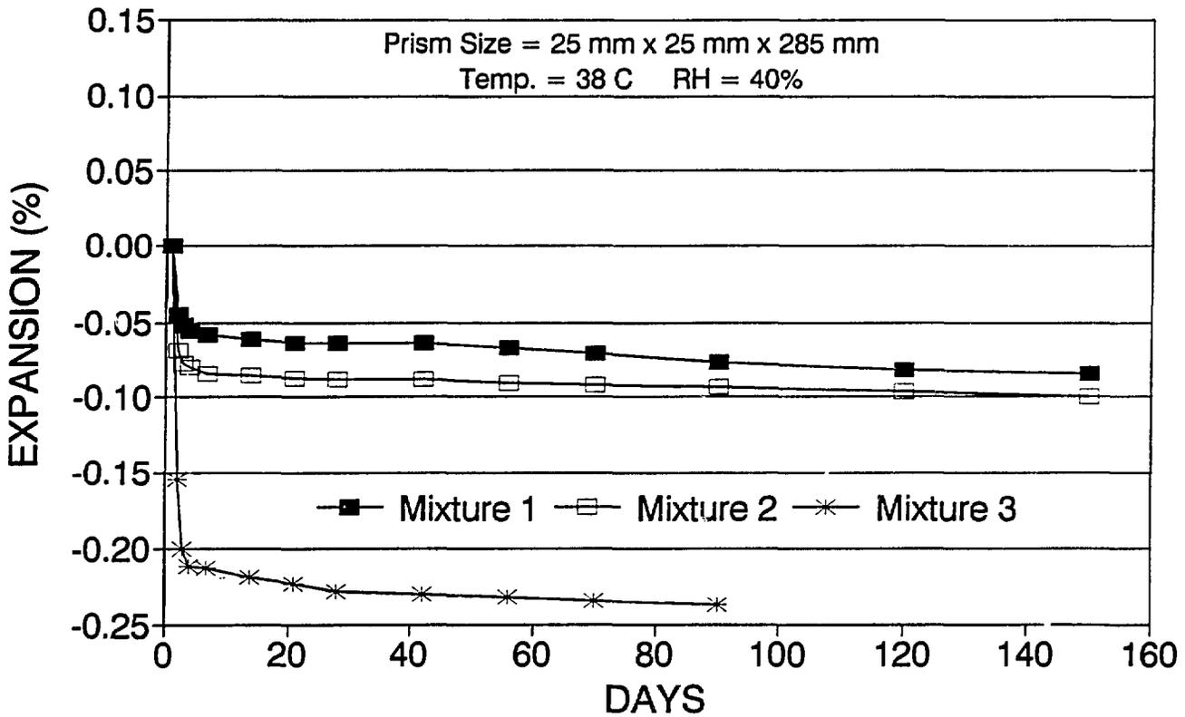
FIGURE 3. HANFORD COLD CAP VOLUME STABILITY VS TIME
