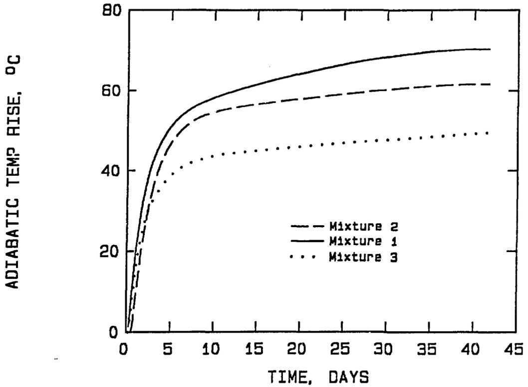
FIGURE 4. HANFORD COLD CAP CALCULATED ADIABATIC TEMPERATURE RISE
