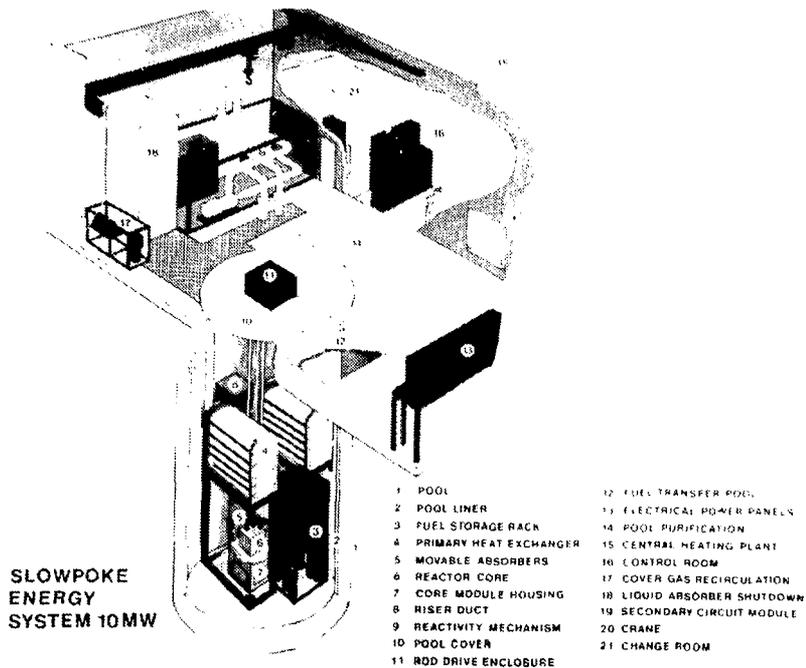
**FIGURE 3: Cutaway View of the 10 MW SLOWPOKE Energy System as a Commercial Installation**
