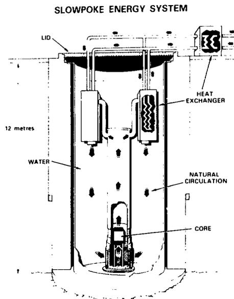
FIGURE 1: Schematic Diagram of the SLOWPOKE Energy Concept
